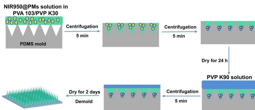
**Figure S3.** Schematic illustration of the fabrication process of NIR950@PMs@MN. PDMS: polydimethylsiloxane.
