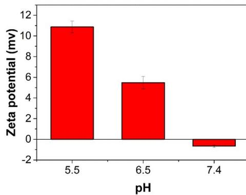
**Figure S5.** Zeta potential of NIR950@PMs incubated in buffers at different pH values at 37°C (Mean  $\pm$  SD,  $n = 3$ ).
