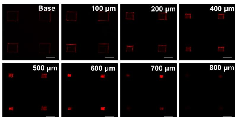
**Figure S4.** CLSM images of cross sections of Cancer Yellow@MN obtained at different heights ( $\lambda_{exc} = 488 \text{ nm}$ , Scale bar:  $200 \mu\text{m}$ ).
