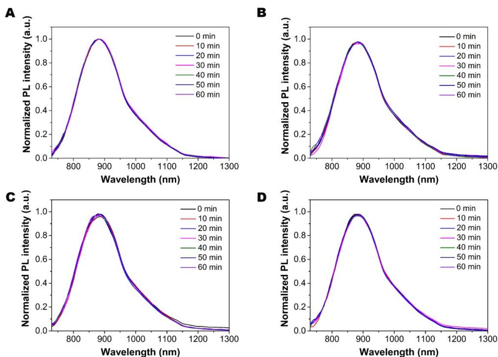
**Figure S1.** Photoluminescence spectra of NIR950@PMs in DI water under continuous 808 nm laser irradiation at (A) 1 W/cm<sup>2</sup>, and (B) 0.35 W/cm<sup>2</sup>, (C) PBS with pH = 6.5 under continuous 808 nm laser irradiation (1 W/cm<sup>2</sup>), (D) PBS with pH = 5.5 under continuous 808 nm laser irradiation (1 W/cm<sup>2</sup>). ( $\lambda_{ex} = 700$  nm).
