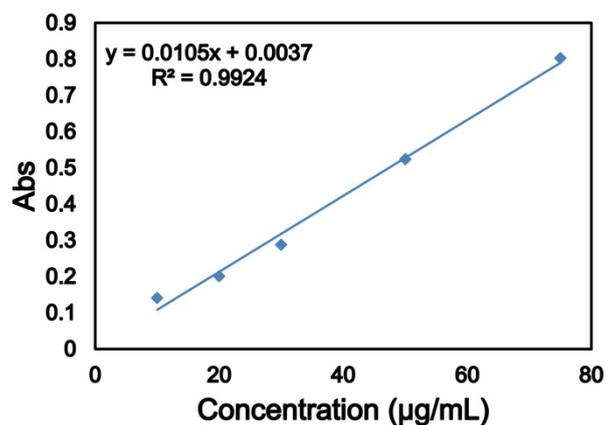
**Figure S2.** The linear relationship between UV absorbance and concentrations of NIR950 in ethanol solution ( $R^2 = 0.9924$ ).
