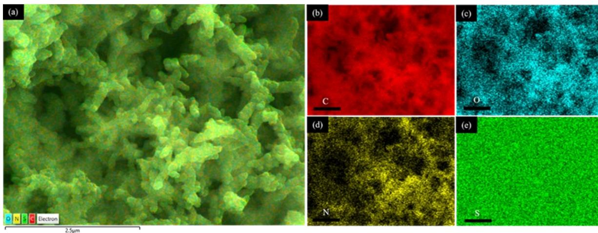
Figure. S3. FE-SEM image of the protonated emeraldine salt of s-PANINbs (a) and the corresponding elemental color mapping of carbon (C-K) (b), oxygen (O-K) (c), nitrogen (N-K) (d), and sulfur (S-K) (e).
