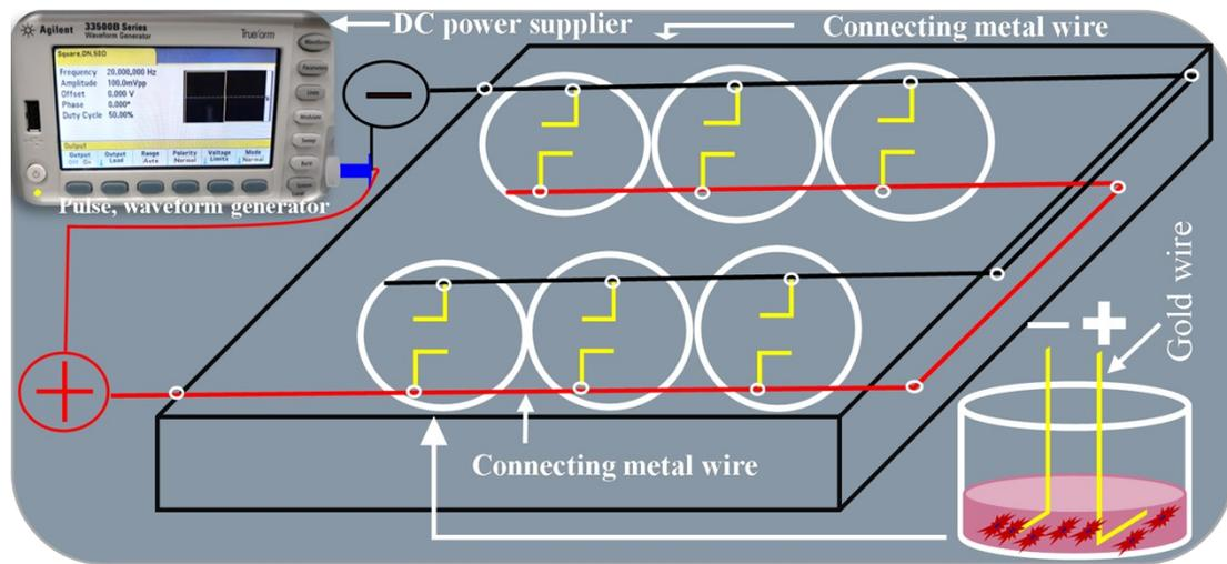
Figure. S2. Schematic representation of in vitro cell culture to promote PC12 cell proliferation and differentiation under electrical stimulation. 12- well plate was used to design of electrical device.
