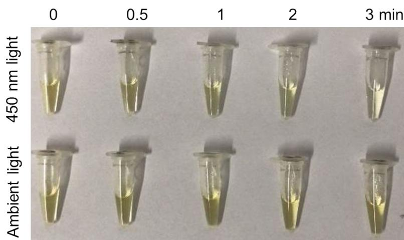
**Fig. S3** Pictures of STX extract exposed to 450 nm light and ambient light at different time intervals. Light irradiation condition:  $0.10 \text{ W cm}^{-2}$ .
