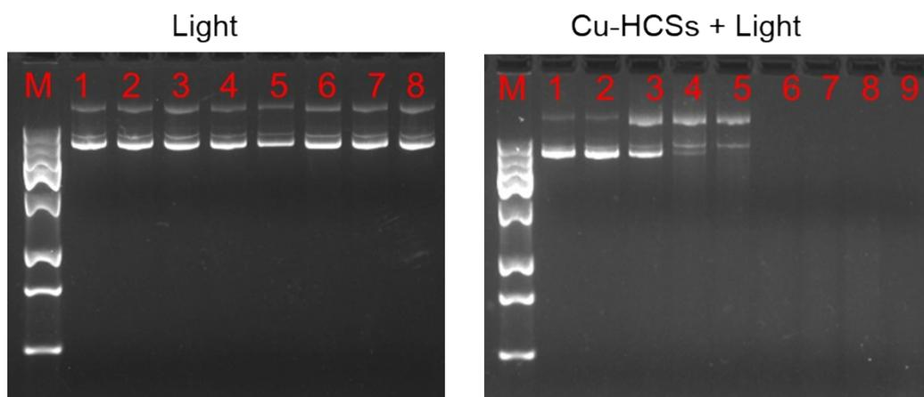
**Fig. S6** Plasmid DNA photocleavage with/without Cu-HCSs at different irradiation time of light. For light-treated group only, M: molecular marker; 1: DNA, 2-8: L (1, 3, 6, 9, 12, 15, 30 min, respectively). For Cu-HCSs/light-treated group, M: molecular marker; 1: DNA; 2-7: Cu-HCSs + L (0, 1, 3, 6, 9, 12, 15, 30 min, respectively). [Cu-HCSs] =  $200 \mu\text{g mL}^{-1}$ , power density of light (450 nm) =  $0.55 \text{ W cm}^{-2}$ .
