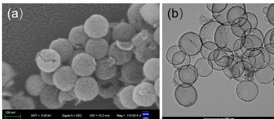
**Fig. S1** SEM image (a) and TEM image (b) of Cu-HCSs.
