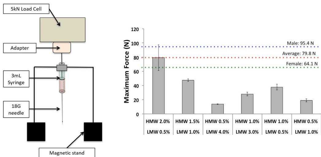
**Supplemental Figure 5c:** A customised injection force rig was used to make measurements of the maximum force required to inject hydrogels through a syringe (3mL Luer-Lock syringe, 18G needle). The average maximum injection force for males, females and both genders combined are depicted as the dotted blue, green and red lines respectively.
