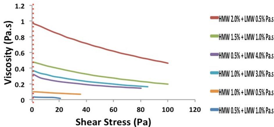
**Supplementary Figure 5a:** Shear thinning curve of pre-gel solutions. The pre-gel viscosity was determined from the curves lowest point of stress.
