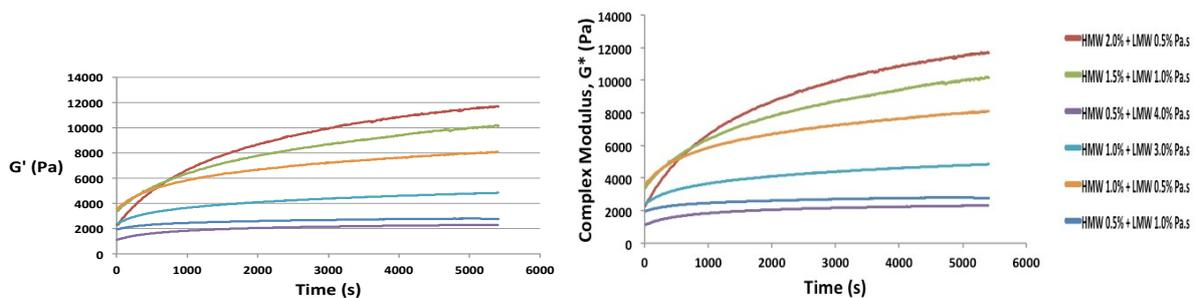
**Supplementary Figure 5b:** Rheological time sweep of crosslinked hydrogels, confirming gelation and comparing the elastic ( $G'$ ) and storage ( $G''$ ) modulus
