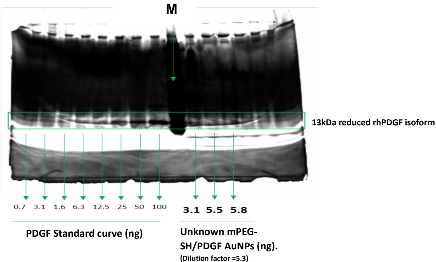
**Supplementary figure 3.** Silver staining of mPEG-SH/PDGF AuNPs. PDGF conjugated AuNPs were produced by standard methods and analysed by SDS-PAGE and Silver staining. Left side: PDGF standard curve (range 0.7-100 ng); M: Marker lane; Right side: PDGF bound to mPEG-SH/PDGF AuNPs. Gel images were acquired with a Amersham GelDoc system and standard curve was generated and analysed using the standard curve tool in Image Lab (Biorad).
