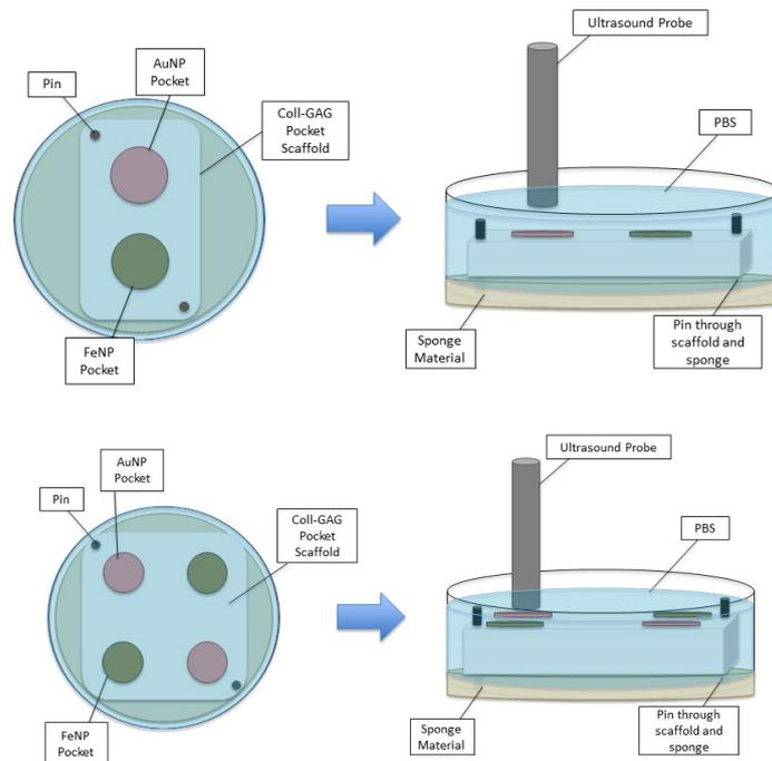
**Supplementary figure 6:** Ultrasound release study setup for (A) Two Pocket Collagen-GAG Scaffold and (B) Four Pocket Collagen-GAG Scaffold
