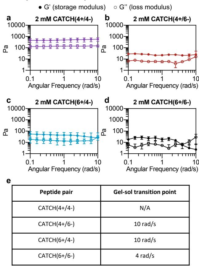
**Figure S1. Oscillating rheology of 2 mM CATCH(+-) hydrogels.** (a-d) Storage and loss modulus of 2 mM CATCH(4+/4-), CATCH(4+/6-), CATCH(6+/4-), and CATCH (6+/6-) at different angular frequencies. The filled circles correspond to the storage modulus and the open circles to the loss modulus. (e) Frequency at which the gel stops behaving as a viscoelastic solid and behaves as a liquid ("gel-sol transition point"). Data are presented as the mean  $\pm$  standard deviation ( $n = 3$ ).
