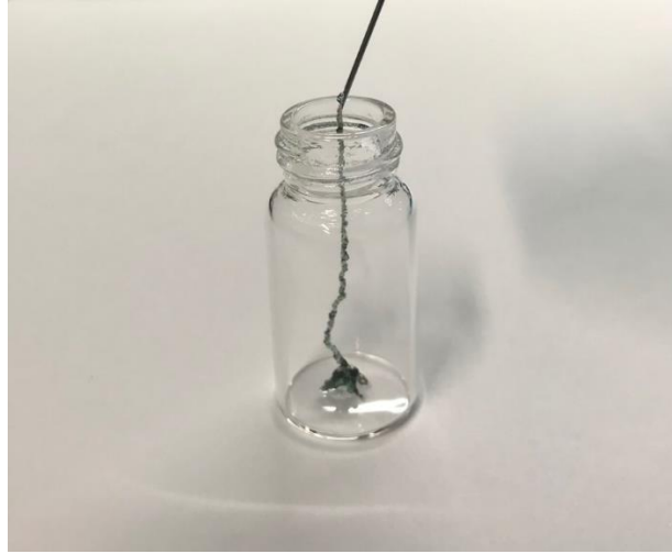
Fig. S1. Injectability test of HC/Cu/ICG8 gel with a single syringe.
