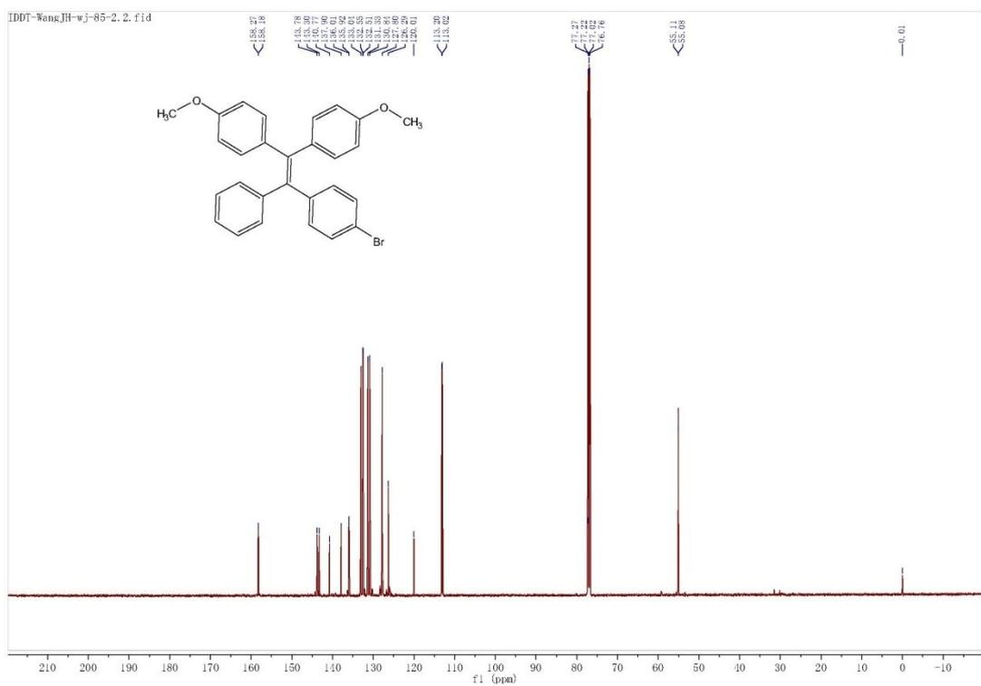
Figure S3.  $^{13}\text{C}$  NMR spectrum of compound 1 (126 MHz, Chloroform-d).
