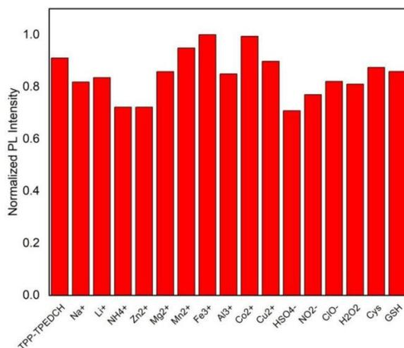
**Figure S22.** Fluorescence intensity (at 626 nm) of TPP-TPEDCH upon addition of 10 eq. various analytes in 99% PBS/DMSO solution. Compound concentration: 20  $\mu$ M. Analytes concentration: 200  $\mu$ M.
