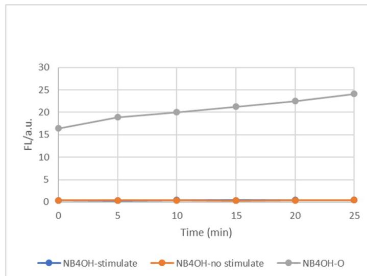
Figure S4: Photostability of NB4OH (20 μM) in DMSO-BB in the absence (orange spot) and present (blue spot) of an xenon lamp irradiated for 25 min, and fluorescence intensity of NB4OH in the presence of NaClO (grey spot) irradiated by an xenon lamp for 25 min(ex=460nm,em=540nm).
