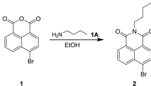
To a solution of compound **1** 4-Bromo-1,8-naphthalic anhydride (5.00 g, 18.1 mmol) in EtOH (50.0 mL) was added compound **1A** Butylamine (1.32 g, 18.1 mmol). The mixture was stirred at 78 °C for 12 hours. The mixture was concentrated under reduced pressure. The mixture was purified by silica gel column chromatography (Petroleum ether: EtOAc = 10:1) to afford compound **2** (3.00 g, 9.03 mmol, 50.0% yield) as a light green solid.
