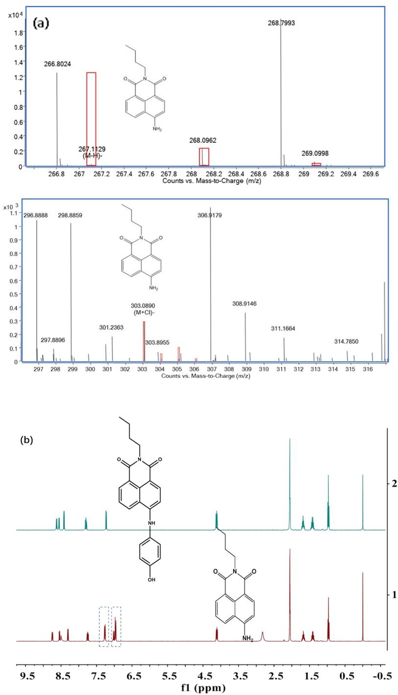
Figure S7: (a)The mass spectrum from the reaction of NB4OH and NaClO in deionized water.
