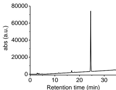
**Fig. S6.** Chromatogram of EROH (retention time = 24.5 min). The chromatogram was monitored at 254 nm with methanol (flow rate, 0.6 mL/min) and water (flow rate, 0.4 mL/min) containing 0.1% trifluoroacetic acid as eluents.
