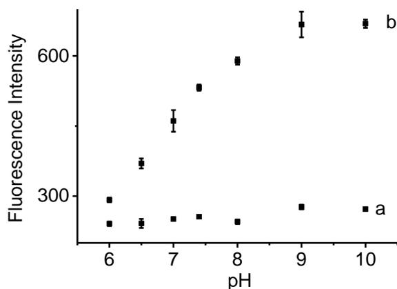
**Fig. S9** Effects of pH on the fluorescence intensity of (a) EROH (1  $\mu\text{M}$ ) and (b) its reaction system with Fenton reagent (500  $\mu\text{M}$   $\text{Fe}^{2+}$ -EDTA + 500  $\mu\text{M}$   $\text{H}_2\text{O}_2$ ) in PBS.  $\lambda_{\text{ex/em}} = 385/446$  nm.
