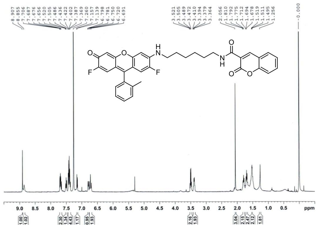
Fig. S3  $^1\text{H}$  NMR spectrum of EROH (400 MHz,  $\text{CDCl}_3$ , 298 K).
