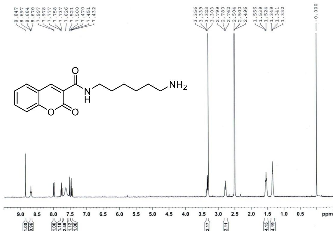
**Fig. S1** <sup>1</sup>H NMR spectrum of CCA-hexanediamine (400 MHz, DMSO-*d*<sub>6</sub>, 298 K).
