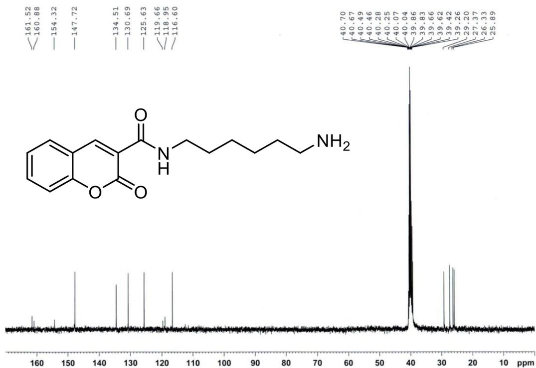
Fig. S2  $^{13}\text{C}$  NMR spectrum of CCA-hexanediamine (100 MHz, DMSO- $d_6$ , 298 K).
