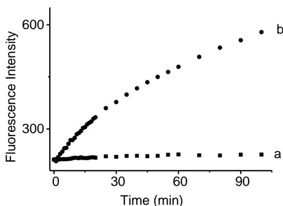
**Fig. S8** Time-course curves of the fluorescence change of EROH (1  $\mu\text{M}$ ) in the absence (a) and presence (b) of Fenton reagent (500  $\mu\text{M}$   $\text{Fe}^{2+}$ -EDTA + 500  $\mu\text{M}$   $\text{H}_2\text{O}_2$ ).  $\lambda_{\text{ex/em}}=385/446$  nm.
