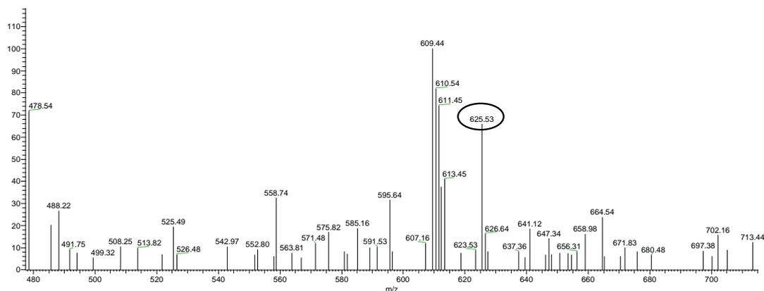
**Fig. S7** ESI mass spectrum of the reaction solution of probe EROH (1  $\mu\text{M}$ ) with Fenton reagent. The peak at  $m/z = 625.53$  indicates the generation of hydroxylation product of the probe; however, the attempt to separate out the hydroxylation product by HPLC-MS was failed due to the low reaction yield of  $< 5\%$  as reported previously.<sup>S3</sup>
