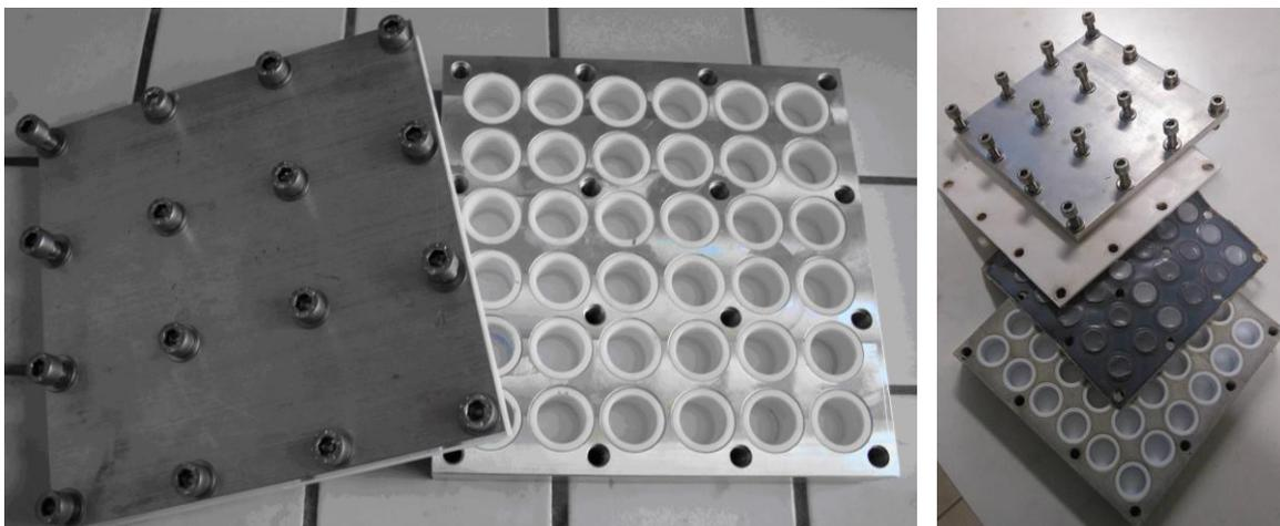
**Figure S1.** Image of the high-throughput system that was used for the hydrothermal syntheses.
