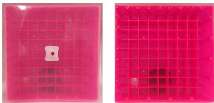
**Figure S7** “Home-made” gas chamber with 81 units for the analysis of the filter paper discs impregnated with  $[1.3\text{Cu}^{2+}]^{3+}$ .
