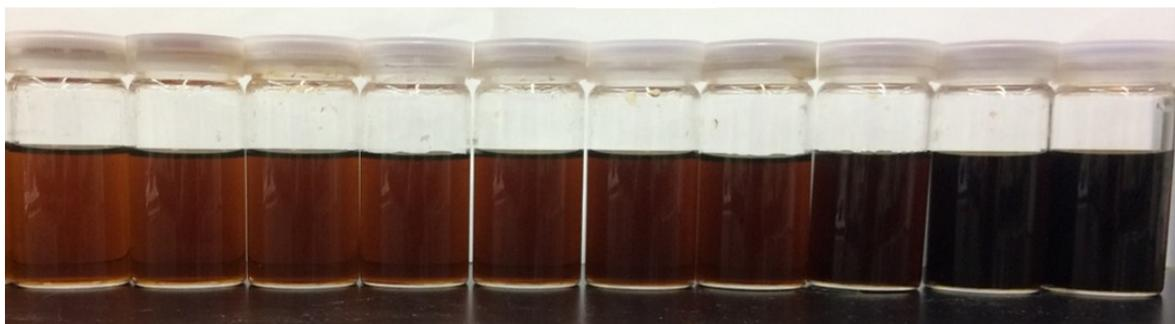
**Figure S1.** The color changes of the GO dispersions under acidic and basic conditions (pH = 2-11).
