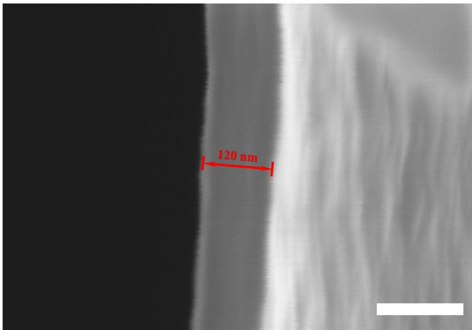
**Figure S1. Cross profile of the thin Au foil. Scale bar: 150 nm.**
