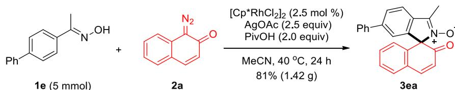
A mixture of oximes (**1e**, 5 mmol), diazo compounds (**2a**, 7.5 mmol),  $[\text{Cp}^*\text{RhCl}_2]_2$  (2.5 mol %), AgOAc (2.5 equiv), PivOH (2.0 equiv) and MeCN (50 mL) were charged into a oven-dried seal-tube. The reaction mixture was stirred under  $\text{N}_2$  at 40 °C for 24 h. After the solvent was removed under reduced pressure, the residue was purified by silica gel chromatography using petroleum ether/ethyl acetate (1:1) to afford the product **3ea** (1.42g, 81%) as a brown solid.
