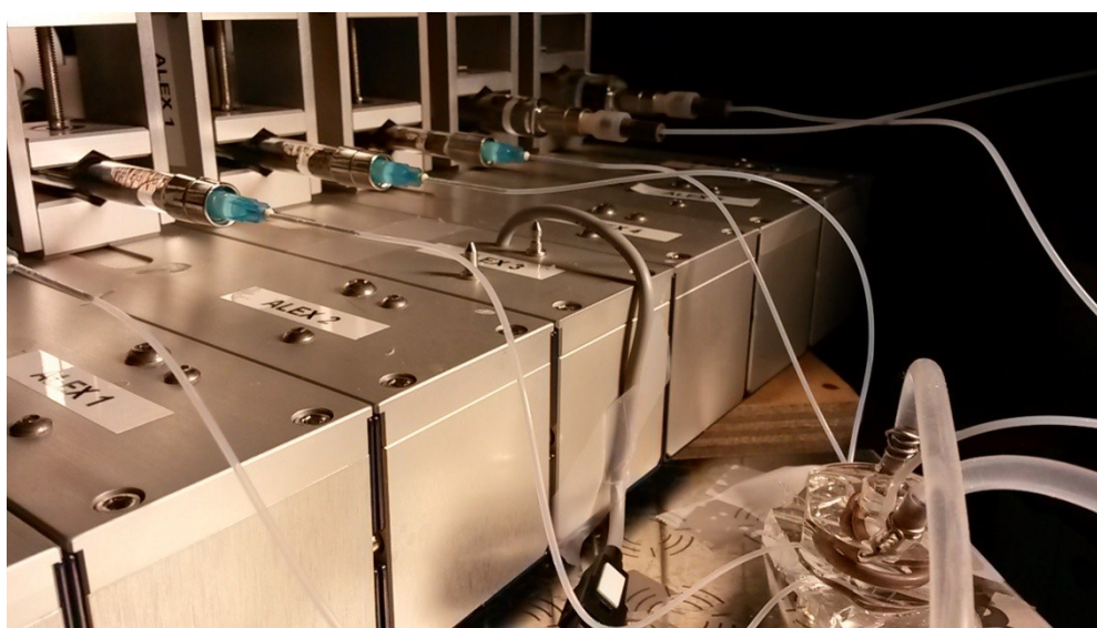
Figure S1: Setup of a typical CSTR experiment. Syringes are mounted on pumps with four of the six syringes depicted connected to the CSTR via inlet tubing and the remaining two used for detection in the microfluidics chip (not shown here). The outlet tubing is either connected to a fraction collector or a microfluidics chip. The CSTR made of PDMS, with the outlet tubing on the right and the four inlets on the left. A copper tube, which is connected to a thermostatic water bath, encircles the CSTR (without making contact with the contents of the CSTR), enables control over the temperature of the CSTR. A
