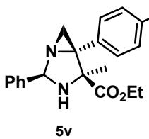
Following the typical procedure, the reaction of 3-(*p*-Fluorobencene)-2*H*-azirine (20.2 mg, 0.15 mmol) and **3a** (41.1 mg, 0.20 mmol) afforded, after purification by silica gel flash chromatography (cyclohexane-EtOAc 10:1), the cycloadduct **5v** (57.0 mg, 84%, white oil).
