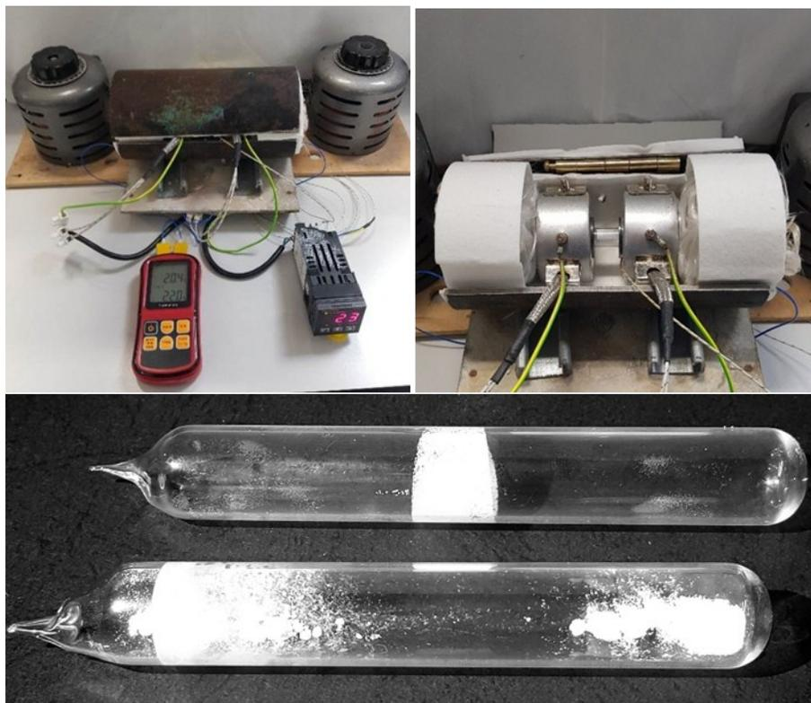
**Fig. S1.** Sublimation apparatus and (lower) sample before sublimation and (upper) cocystal after sublimation.
