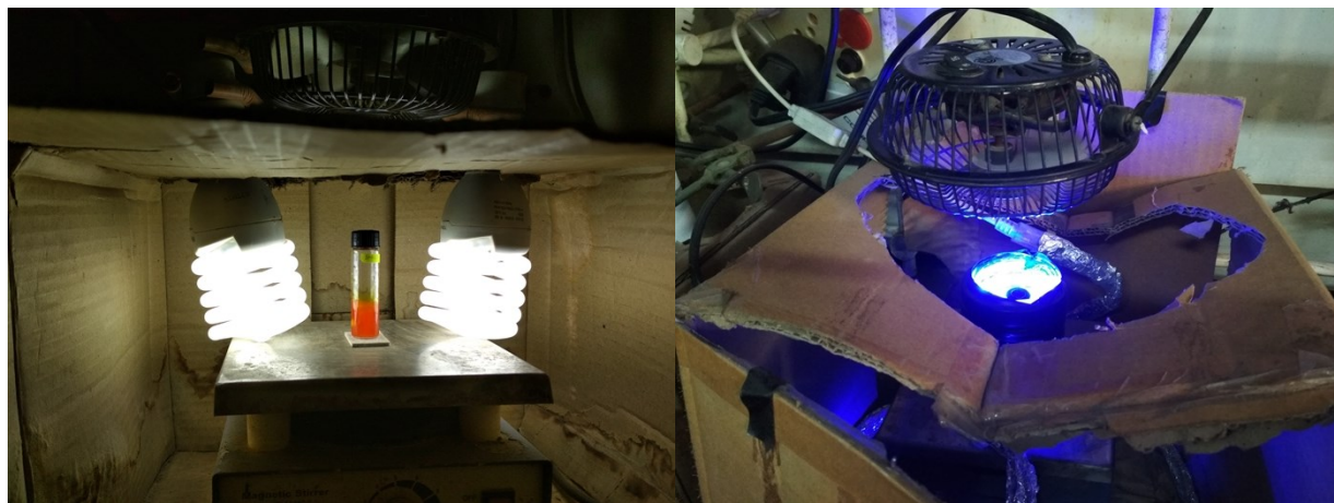
Fig 2: Reaction set-up under CFL (left) and Blue LED strips (right)
