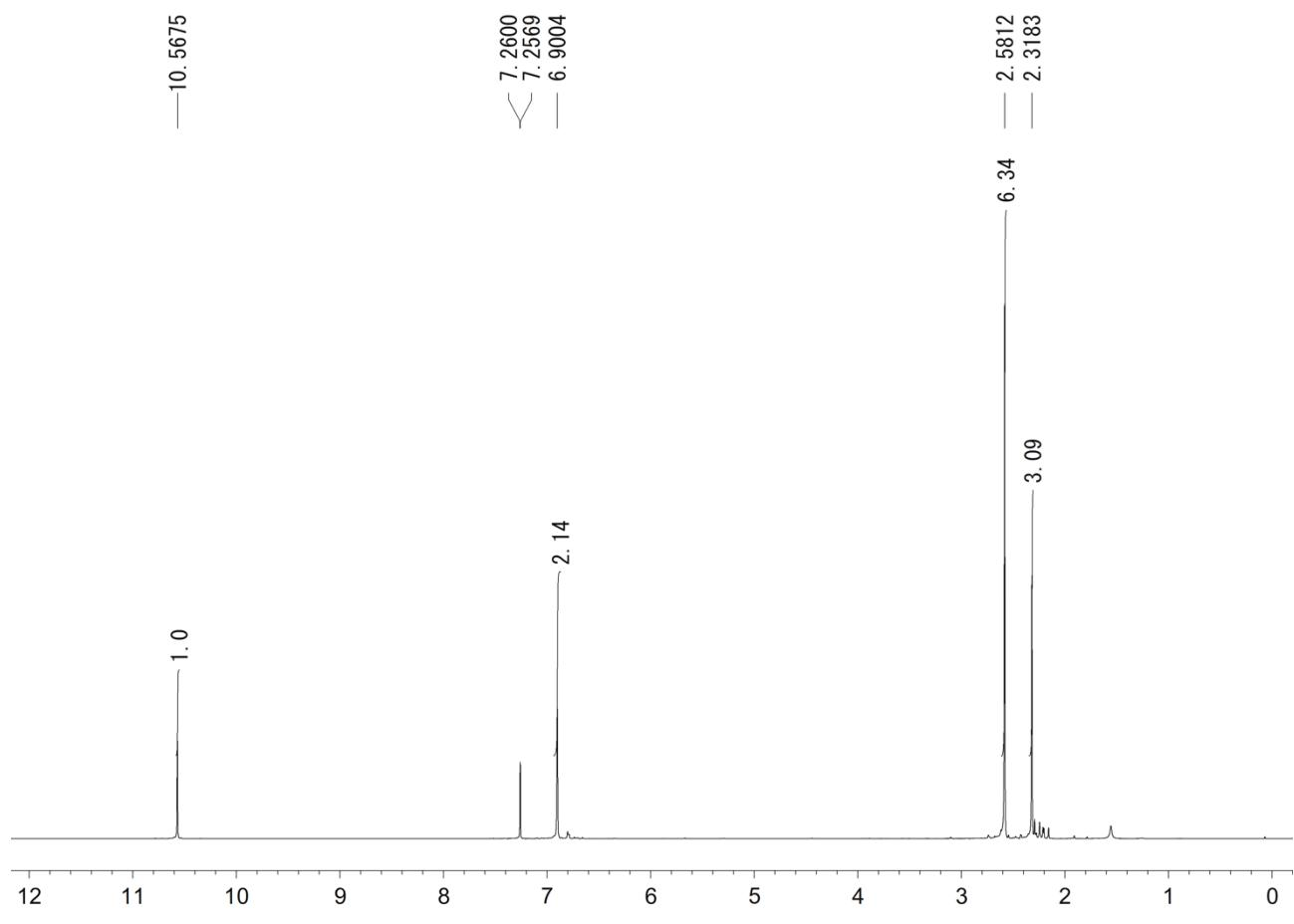
400 MHz  $^1\text{H}$  NMR spectrum of **3d** in  $\text{CDCl}_3$ .
