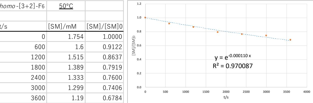
**Fig. S6 Guest-release of *o*-xylene@*homo*-[3+2]-F<sub>6</sub> at various temperatures.**
