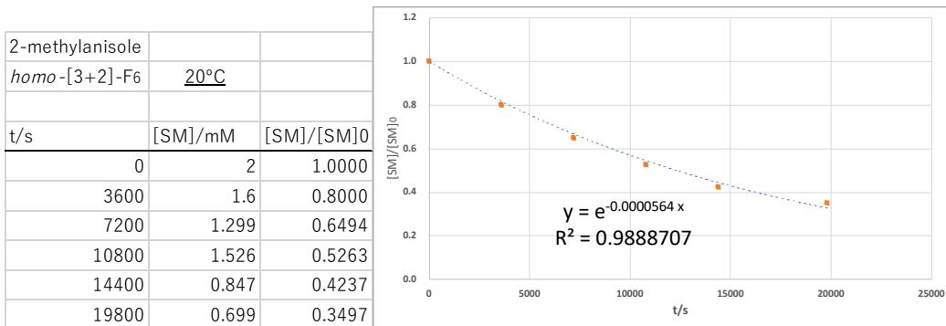
**Fig. S13 Guest-release of 2-methylanisole@*homo*-[3+2]-F<sub>6</sub>.**
