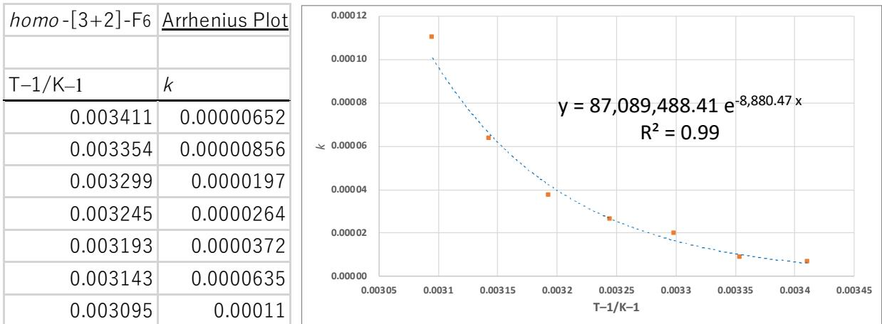
**Fig. S7 Arrhenius plot of guest-release of *o*-xylene@*homo*-[3+2]-F<sub>6</sub>.**
