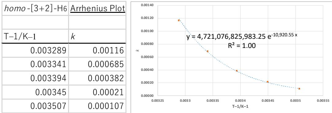
**Fig. S3 Arrhenius plot of guest-release of *o*-xylene@*homo*-[3+2]-H<sub>6</sub>.**
