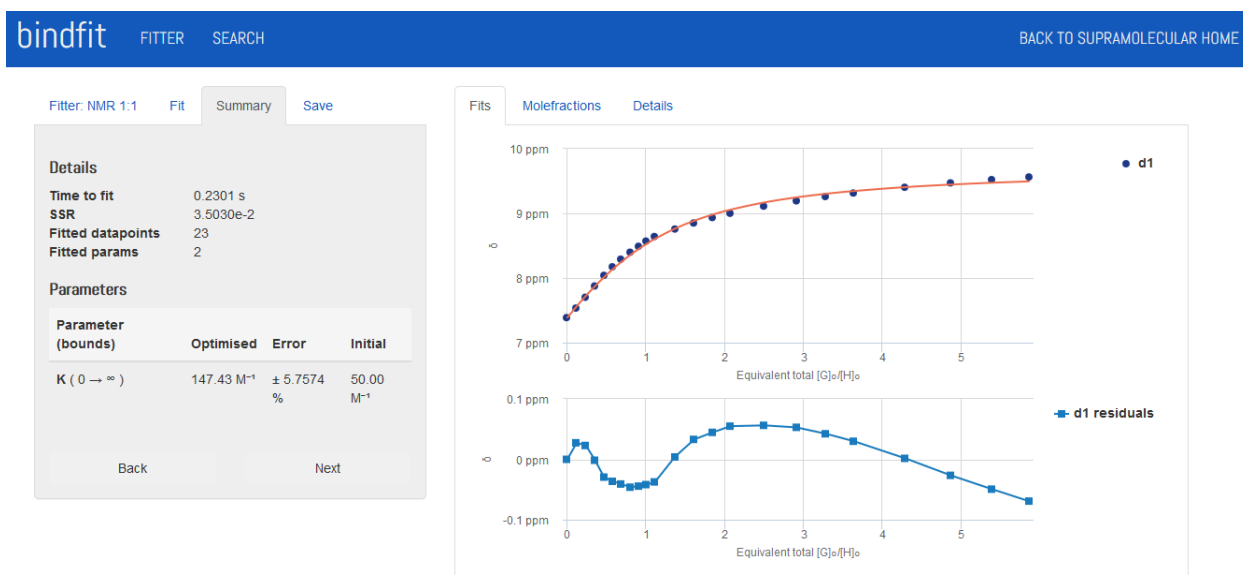
Figure S37: Assessment of binding constant ( K_a ) by ^1\text{H} NMR titration study of 6 (12 mM) with the gradual addition of \text{TBAF} \cdot 3\text{H}_2\text{O} in chloroform- d . 15
