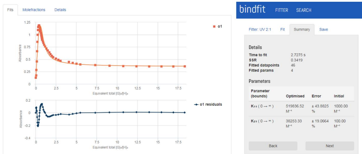
Figure S25: Assessment of binding constant ( K_a ) by UV-vis titration study of 5 (120 \mu\text{M} ) with gradual addition of TBACN in acetonitrile, the absorbance at 396 nm was plotted against cyanide concentration. 13
