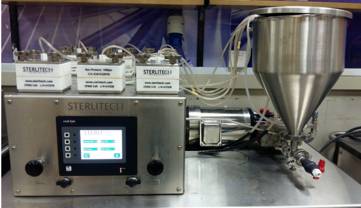
Fig. S5. Schematic illustration of filtration experiment through the cross-flow CF042 cell.
