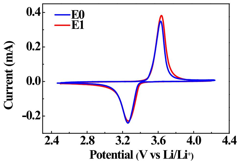
**Figure S1** The cyclic voltammetry (CV) curves of batteries in the E0 and E1 electrolytes.
