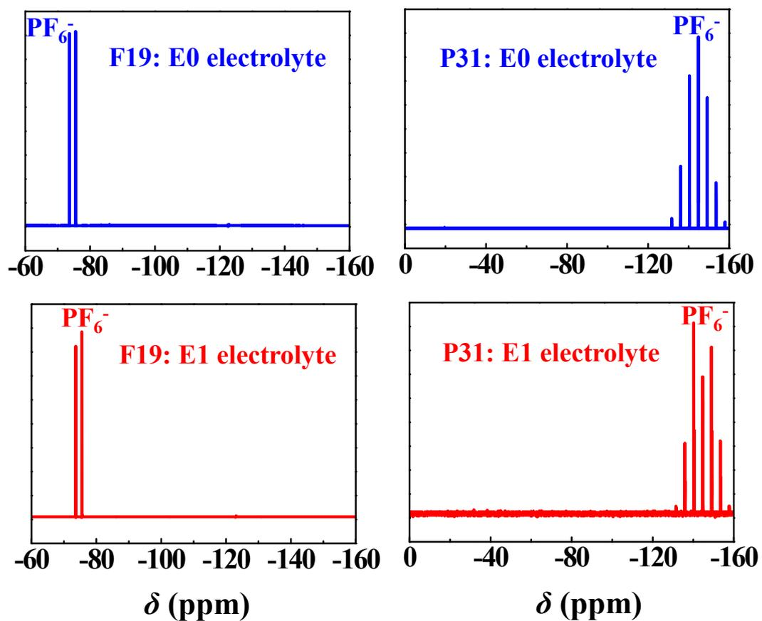
**Figure S8** NMR spectra of the electrolytes with and without CP additive before stored at 80 °C for 48 h.
