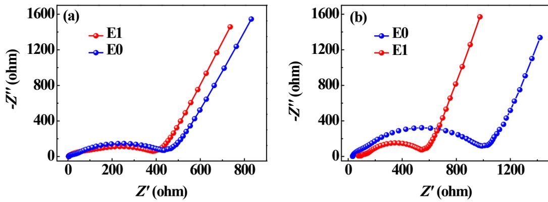
**Figure S2** The electrochemistry impedance spectroscopy (EIS) of batteries in the E0 and E1 electrolytes (a) before and (b) after 200 cycles.
