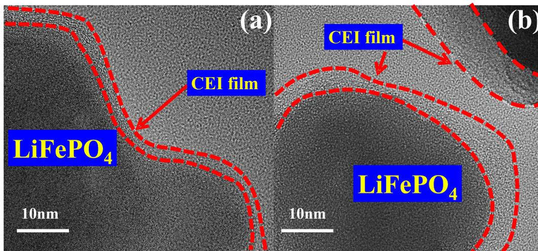
**Figure S6** TEM images of  $\text{LiFePO}_4$  electrodes after 200 cycles at  $60\text{ }^\circ\text{C}$ :
