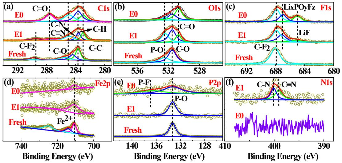
**Figure S7** XPS spectra of electrode materials before and after cycling (E1: with 1 wt.% CP; E0: No additive)
