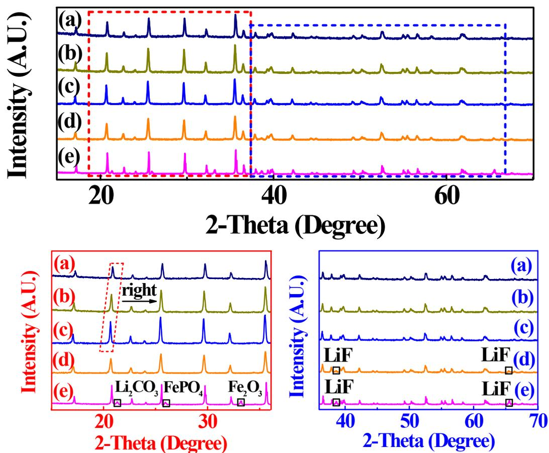
**Figure S5** The XRD patterns of the LiFePO<sub>4</sub> electrode material: stored at 80 °C in the electrolytes (a) without and (b) with CP additive for 48 h; (c) Fresh LiFePO<sub>4</sub>; The electrode materials after 200 cycles in the electrolytes (d) with and (e) without CP at 60 °C.
