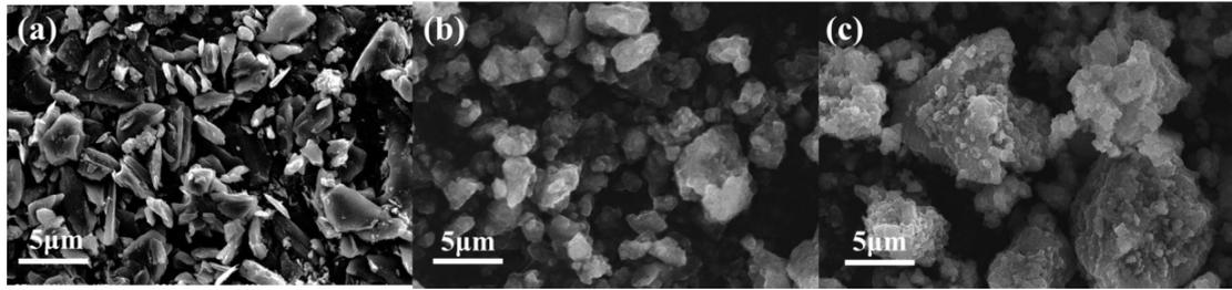
**Figure S4** SEM images of the  $\text{LiFePO}_4$  stored in the electrolytes at  $80\text{ }^\circ\text{C}$  after 24 h: (a) Fresh  $\text{LiFePO}_4$ ;  $\text{LiFePO}_4$  stored in the electrolytes (b) with CP and (c) without CP additive.
