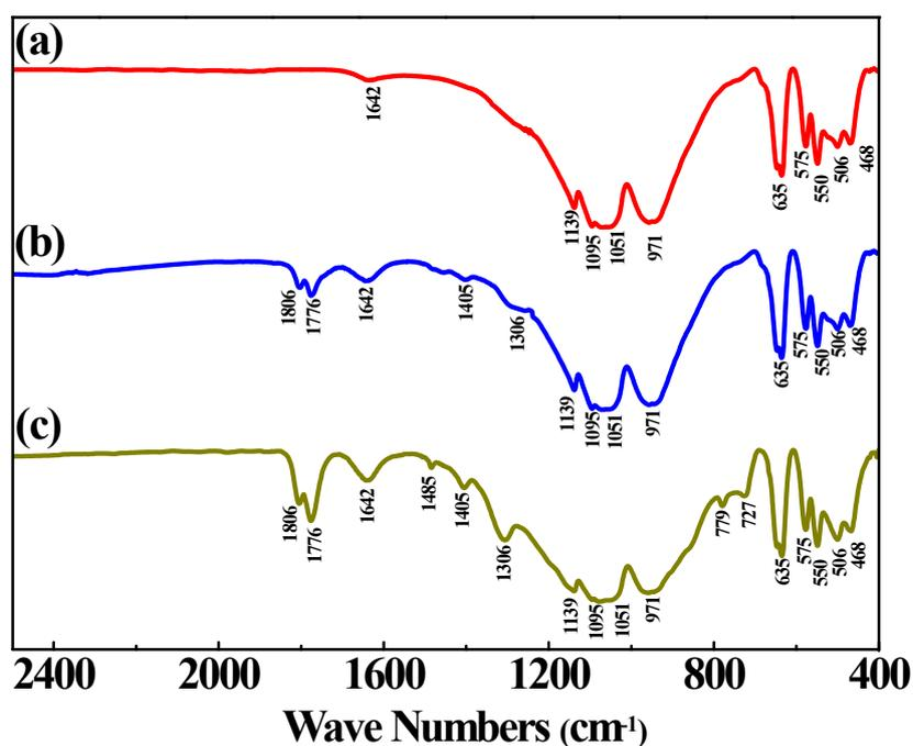
**Figure S3** The FTIR spectra of  $\text{LiFePO}_4$  before and after storage in the different electrolytes: (a) Fresh  $\text{LiFePO}_4$ ;  $\text{LiFePO}_4$  stored at  $80\text{ }^\circ\text{C}$  in the electrolytes (b) with CP and (c) without CP additive for 48 h.
