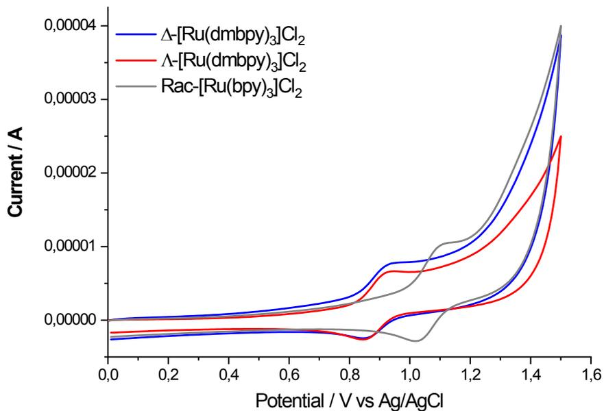
Figure S2. Cyclic voltammograms of 0.5 mM  $\Delta$ -[Ru(dmbpy)<sub>3</sub>]Cl<sub>2</sub>,  $\Lambda$ -[Ru(dmbpy)<sub>3</sub>]Cl<sub>2</sub> and of the racemic [Ru(bpy)<sub>3</sub>]Cl<sub>2</sub> on glassy carbon working electrode in PBS. Scan rate 0.1 V s<sup>-1</sup>.
