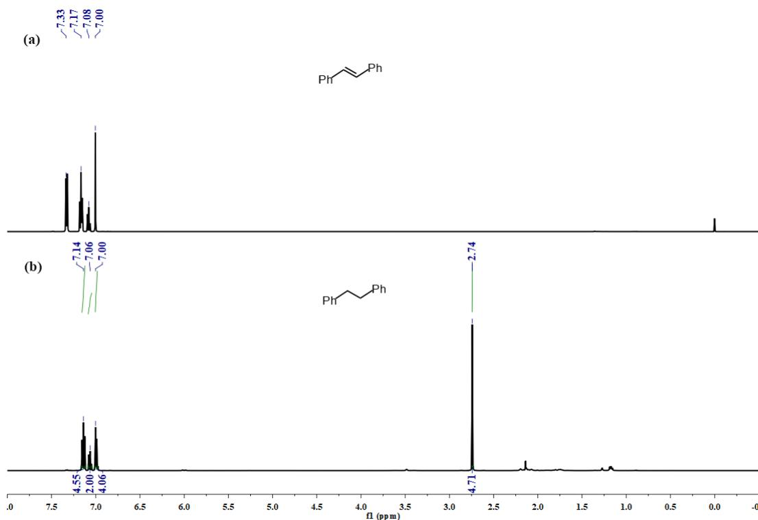
**Figure S24.** Stacked <sup>1</sup>H NMR spectrum (500 MHz, C<sub>6</sub>D<sub>6</sub>, 25 °C) of (a) 1,2-diphenylethylene and (b) 1,2-diphenylethane after catalytic hydrogenation with **2-THP** (5 mol%) and H<sub>2</sub> (10 atm) at 40 °C (entry 4).
