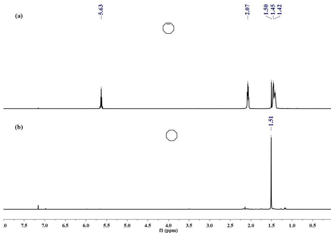
**Figure S31.** Stacked  $^1\text{H}$  NMR spectrum (500 MHz,  $\text{C}_6\text{D}_6$ , 25  $^\circ\text{C}$ ) of (a) cyclooctene and (b) cyclooctane after catalytic hydrogenation with **2-THP** (5 mol%) and  $\text{H}_2$  (10 atm) at 40  $^\circ\text{C}$  (entry 11).
