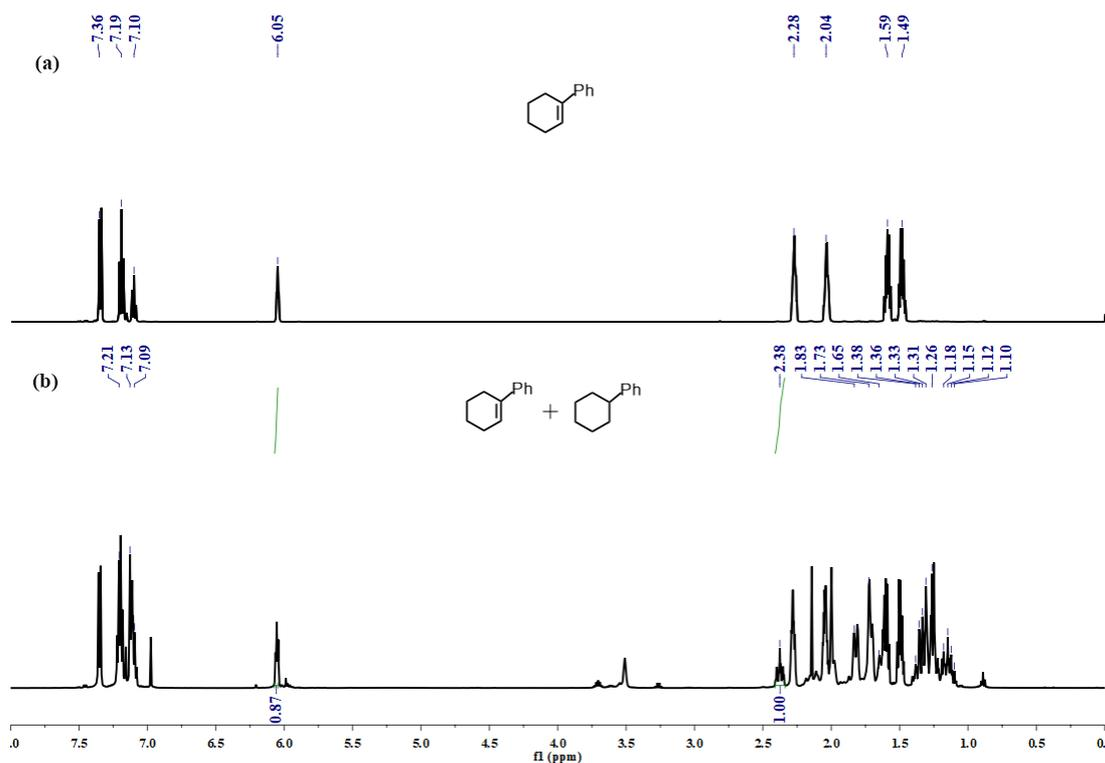
**Figure S25.** Stacked <sup>1</sup>H NMR spectrum (500 MHz, C<sub>6</sub>D<sub>6</sub>, 25 °C) of (a) 1-phenylcyclohexene and (b) 1-phenylcyclohexane after catalytic hydrogenation with **2-THP** (5 mol%) and H<sub>2</sub> (10 atm) at 40 °C (entry 5).
