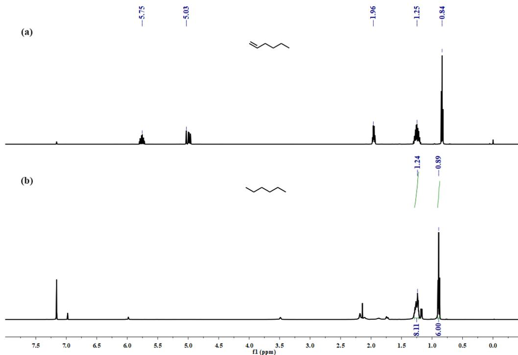
**Figure S27.** Stacked  $^1\text{H}$  NMR spectrum (500 MHz,  $\text{C}_6\text{D}_6$ , 25  $^\circ\text{C}$ ) of (a) 1-hexene and (b) hexane after catalytic hydrogenation with **2-THP** (5 mol%) and  $\text{H}_2$  (10 atm) at 40  $^\circ\text{C}$  (entry 7).
