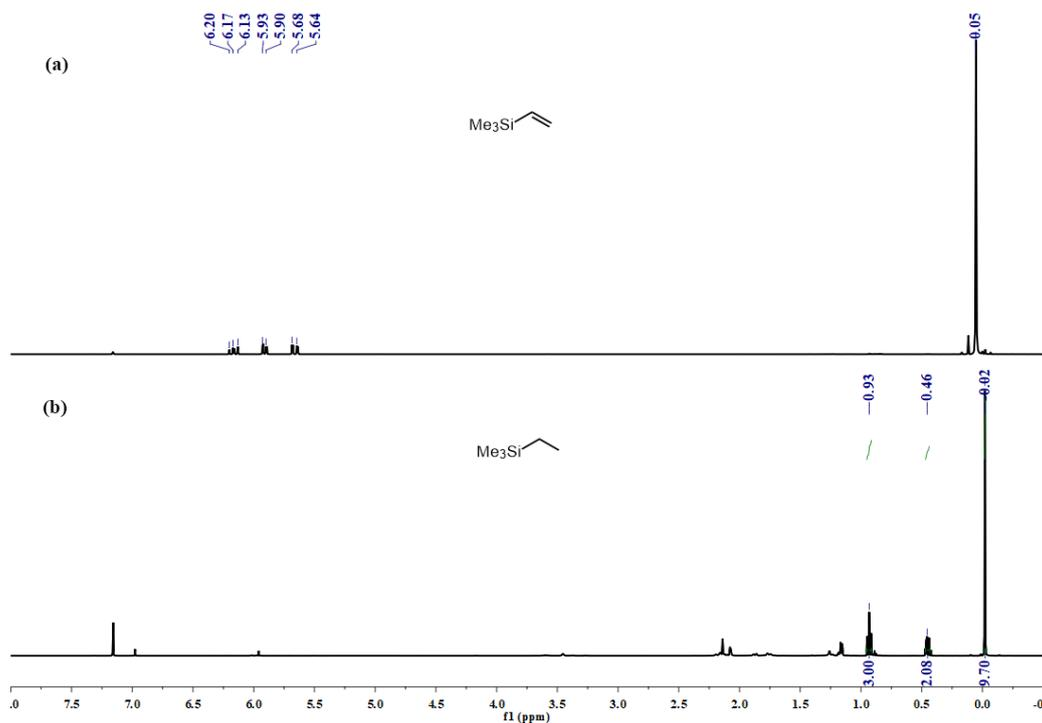
**Figure S26.** Stacked <sup>1</sup>H NMR spectrum (500 MHz, C<sub>6</sub>D<sub>6</sub>, 25 °C) of (a) trimethylsilylethylene and (b) trimethylsilylethane after catalytic hydrogenation with **2-THP** (5 mol%) and H<sub>2</sub> (10 atm) at 40 °C (entry 6).
