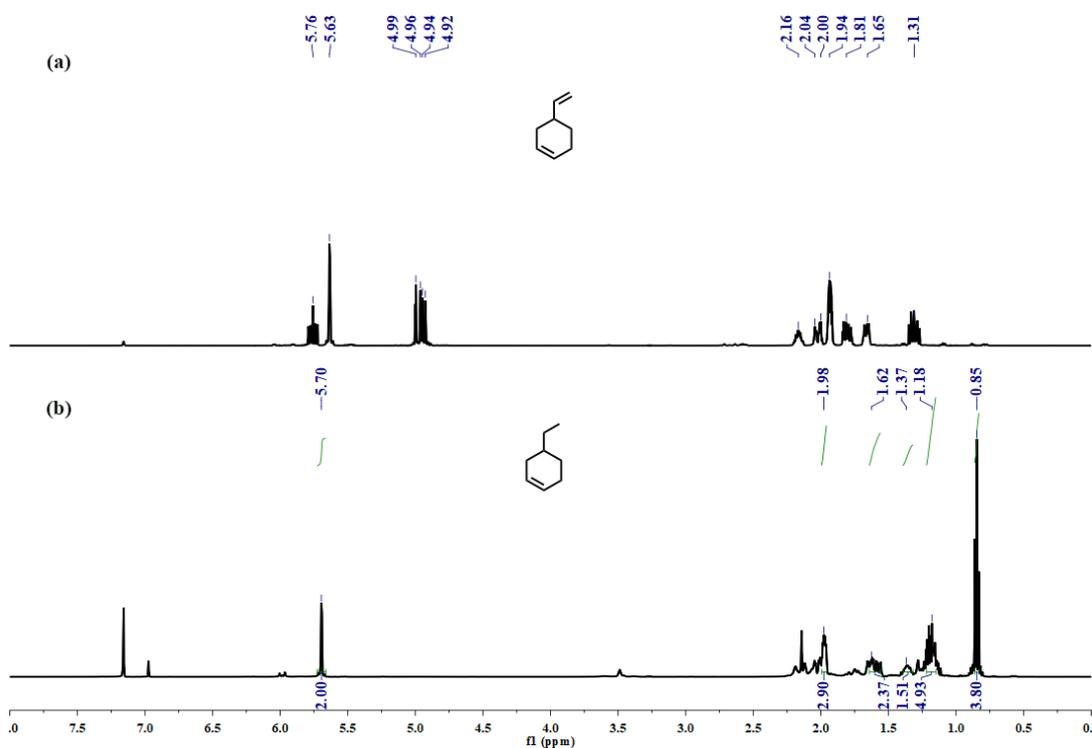
**Figure S32.** Stacked  $^1\text{H}$  NMR spectrum (500 MHz,  $\text{C}_6\text{D}_6$ , 25  $^\circ\text{C}$ ) of (a) 4-ethenylcyclohexene and (b) 4-ethylcyclohexene after catalytic hydrogenation with **2-THP** (5 mol%) and  $\text{H}_2$  (10 atm) at 40  $^\circ\text{C}$  (entry 12).
