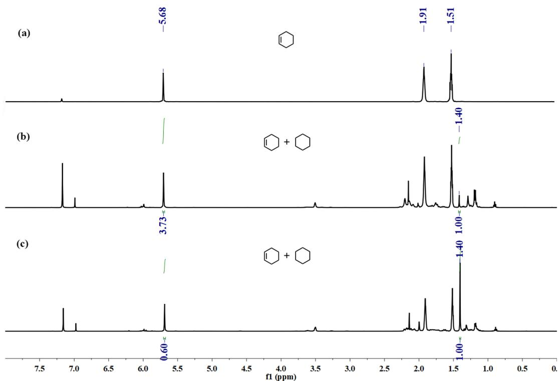
**Figure S33.** Stacked  $^1\text{H}$  NMR spectrum (500 MHz,  $\text{C}_6\text{D}_6$ , 25  $^\circ\text{C}$ ) of (a) cyclohexene and catalytic hydrogenation of cyclohexene mediated by **2-THP** (5 mol%) with  $\text{H}_2$  (10 atm) after (b) 24 hours and (c) 120 hours at 40  $^\circ\text{C}$  (entry 13).
