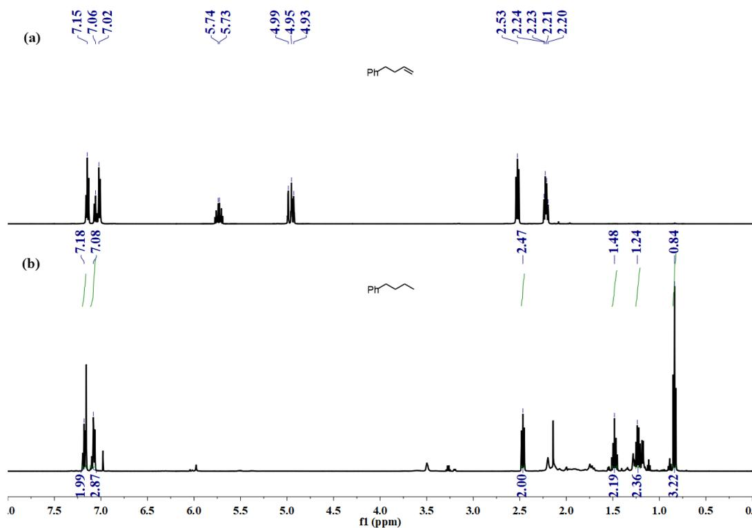
**Figure S28.** Stacked  $^1\text{H}$  NMR spectrum (500 MHz,  $\text{C}_6\text{D}_6$ , 25  $^\circ\text{C}$ ) of (a) 4-phenyl-1-butene and (b) 1-butylbenzene after catalytic hydrogenation with **2-THP** (5 mol%) and  $\text{H}_2$  (10 atm) at 40  $^\circ\text{C}$  (entry 8).
