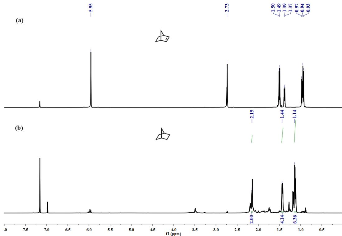
**Figure S30.** Stacked  $^1\text{H}$  NMR spectrum (500 MHz,  $\text{C}_6\text{D}_6$ , 25  $^\circ\text{C}$ ) of (a) norbornene and (b) norbornane after catalytic hydrogenation with **2-THP** (5 mol%) and  $\text{H}_2$  (10 atm) at 40  $^\circ\text{C}$  (entry 10).
