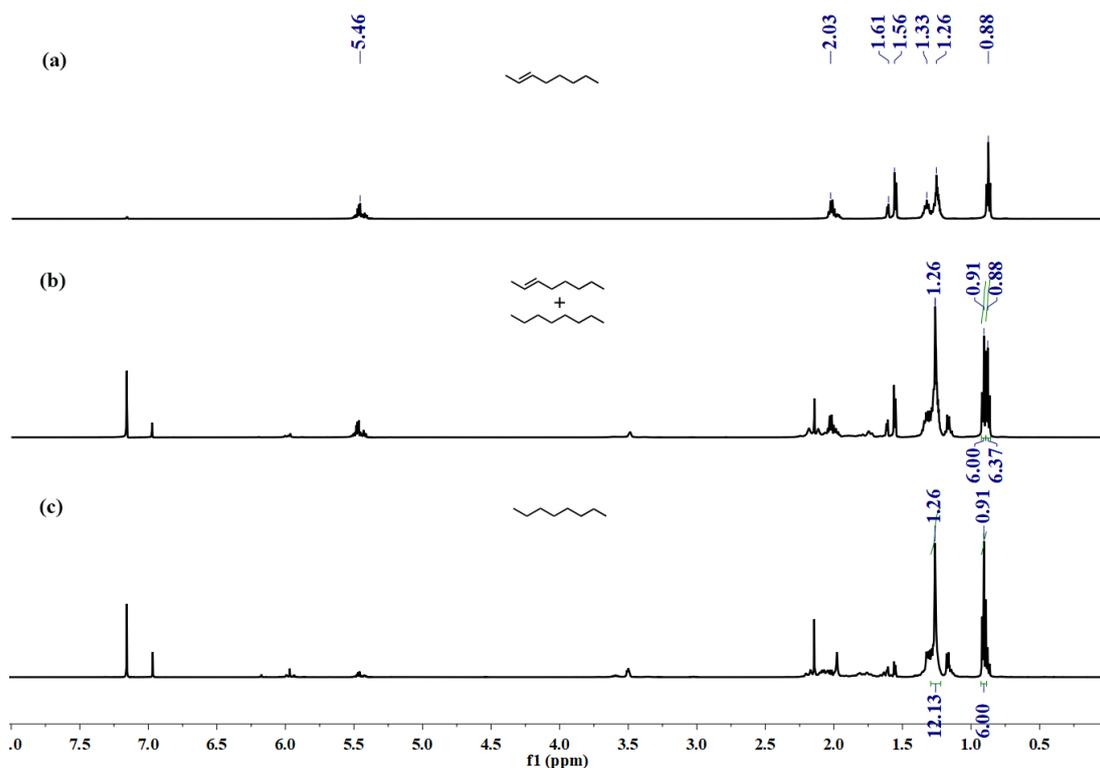
**Figure S29.** Stacked  $^1\text{H}$  NMR spectrum (500 MHz,  $\text{C}_6\text{D}_6$ , 25  $^\circ\text{C}$ ) of (a) 2-octene and catalytic hydrogenation of 2-octene mediated by **2-THP** (5 mol%) with  $\text{H}_2$  (10 atm) after (b) 24 hours and (c) 72 hours at 40  $^\circ\text{C}$  (entry 9).
