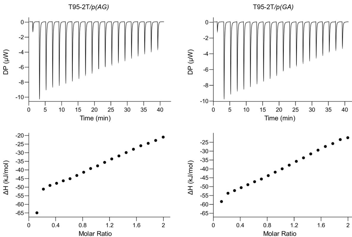
**Figure S4.** ITC binding isotherms of *T95-2T* with *p(AG)* (left) and *p(GA)* (right). *T95-2T*: 5'-TTGGGTGGGTGGGTGGGT-3'. Non-specific binding of the ligands toward *T95-2T* - a parallel G4 without any vacant site.
