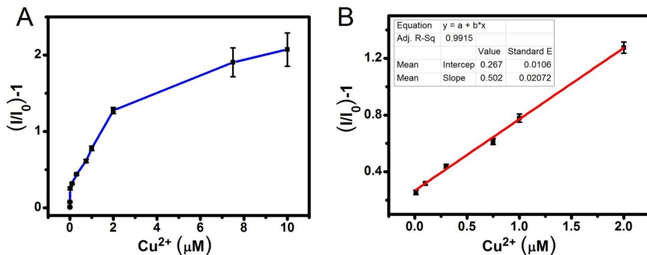
**Fig. S5** The plots (A) and linear responses (B) of  $I_0/I$  ratios against  $\text{Cu}^{2+}$  concentrations. Herein  $I_0$  and  $I$  are the fluorescence intensity at 655 nm in the absence and presence of  $\text{Cu}^{2+}$ , respectively.
