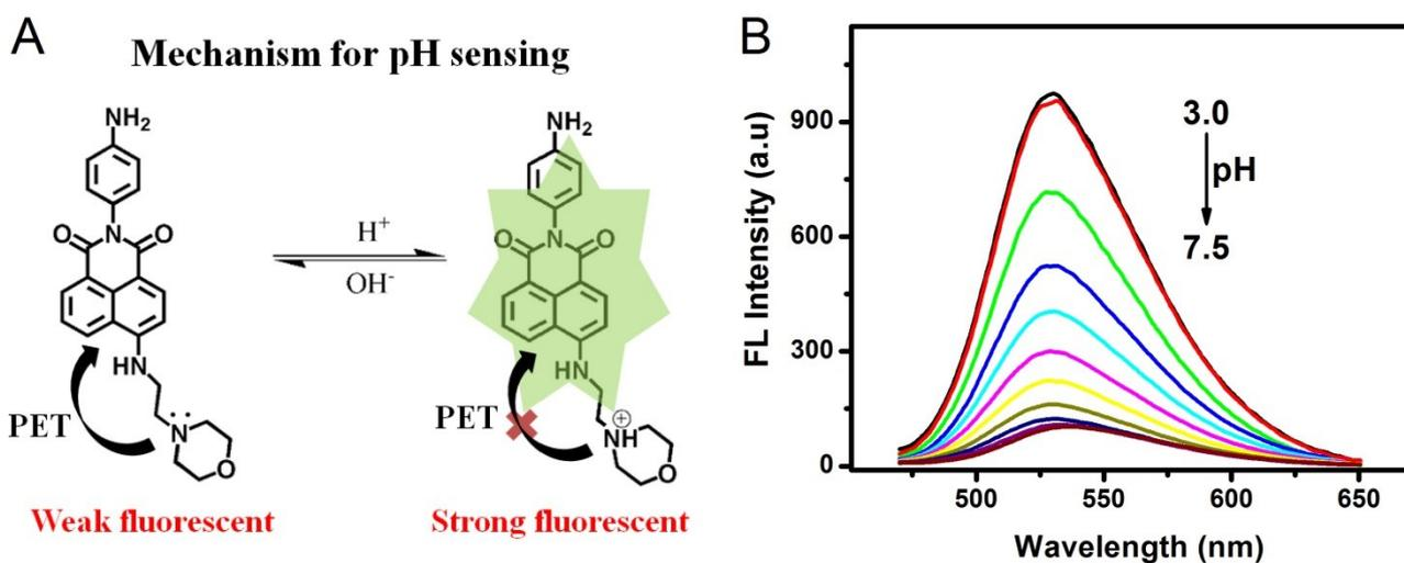
**Fig. S2** (A) Schematic mechanism of NA-NH<sub>2</sub> for pH sensing. (B) Fluorescence responses of NA-NH<sub>2</sub> to various pH values.
