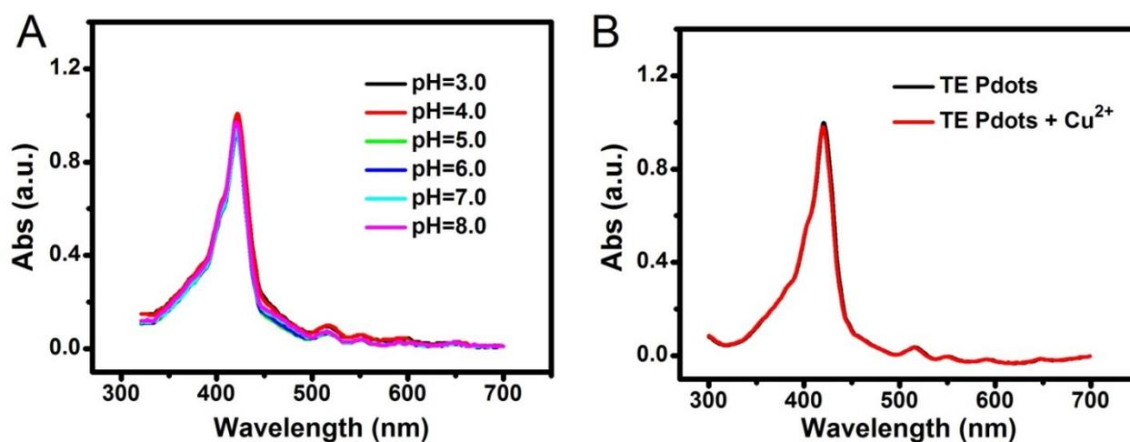
**Fig. S6** UV-vis absorption spectrum of  $4 \mu\text{g mL}^{-1}$  TE Pdots with various pH values (A) and  $20 \mu\text{M}$   $\text{Cu}^{2+}$  (B).
