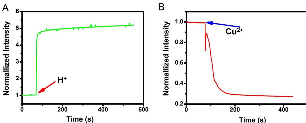
**Fig. S3** Time-dependent fluorescence of TE Pdots ( $4 \mu\text{g mL}^{-1}$ ) recorded at 530 nm for pH (A) and 655 nm  $\text{Cu}^{2+}$  (B) sensing, respectively.
