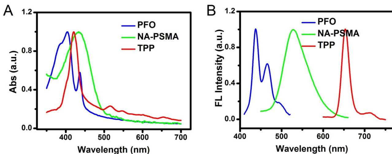
**Fig. S1** UV-vis absorption spectra (A) and fluorescence spectra (B) of PFO (blue line), NA-PSMA (green line) and TPP (red line).
