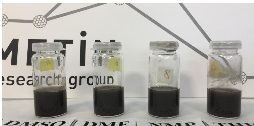
**Figure S3.** Exfoliated BP nanosheets in various solvents (as prepared), from left to right: DMSO, DMF, NMP and THF.
