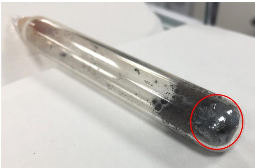
**Figure S2.** A photography of as-prepared BP crystal in the quartz ampoule
