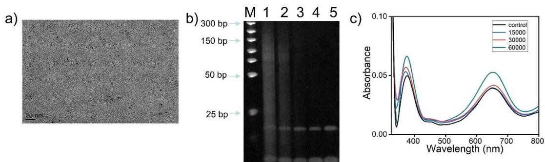
**Figure S3.** (a) TEM image of PtNPs. (b) Conventional PAGE image analysis of extension products: DNA ladder marker (M), telomerase extracts from MDA-MB-231 of 6000 cells (lane 1), 4000 cells (lane 2), 1000 cells (lane 3), 100 cells (lane 4), heated-inactive control (lane 5). (c) UV-vis spectra of MGH catalyzing  $\text{H}_2\text{O}_2$ -mediated oxidation TMB in pH 5.5 buffer ( $\text{H}_2\text{O}_2$  : 50 mM, TMB : 800 mM, Reaction time: 15 min) from different numbers of MDA-MB-231 cell.
