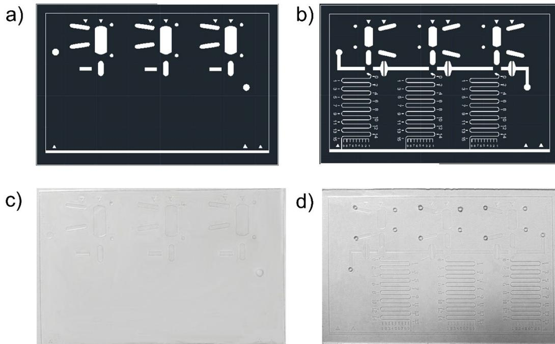
**Figure S2.** Photomasks used for the preparation of TV-Chip (a) Top plate and (b) bottom plate; Images of TV-Chip (c) top plate and (d) bottom plate.
