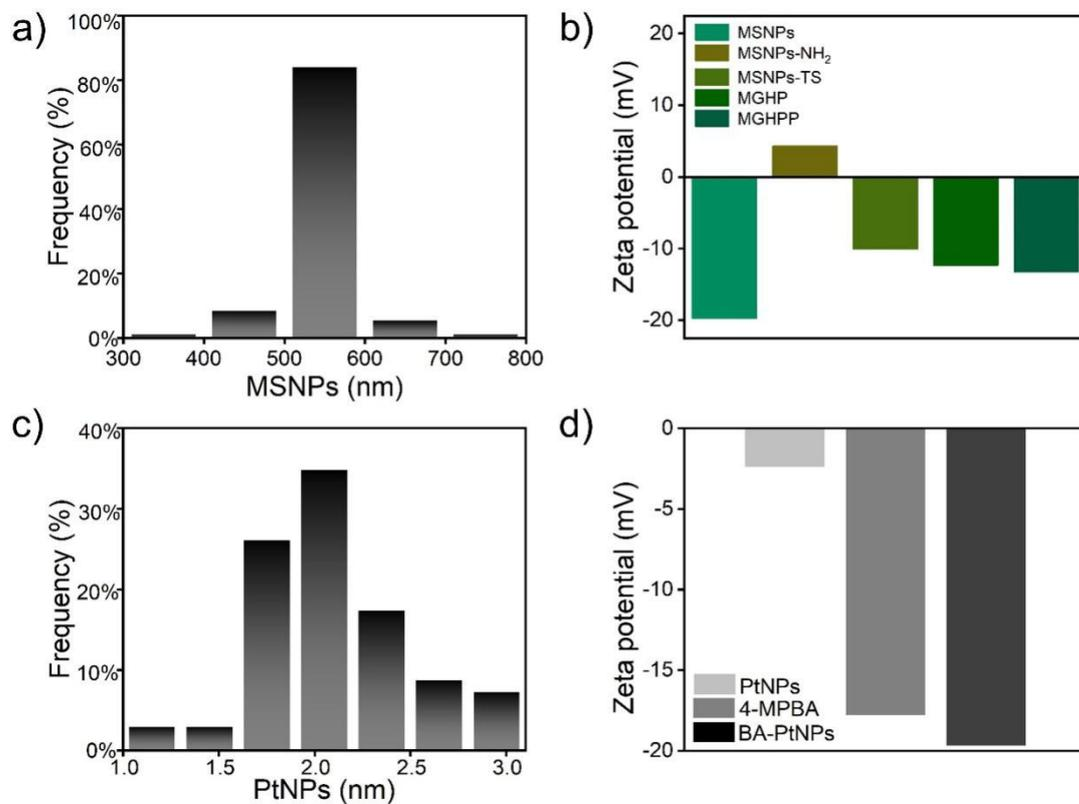
**Figure S1.** (a) Particle size distribution of MSNPs. (b) The Zeta potentials of modified-MSNPs varies with the preparation process. (c) Particle size distribution of PtNPs. (d) Zeta potentials of PtNPs, 4-MPBA, BA-PtNPs.
