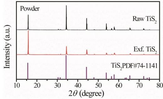
Fig. S2 XRD patterns of Raw- and Exfoli- (Exf.)  $\text{TiS}_2$  powders.
