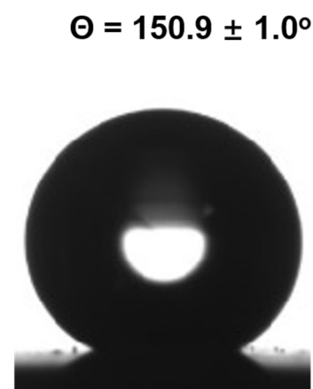
Figure S11. a) Construction of biomimetic superhydrophobic Interface. Silicon surfaces were kept dipped in acidic \text{KMnO}_4 overnight and washed using DI water. Then the silicon surface was kept dipped in 0.01 % \text{NaOH} and \text{HNO}_3 for 10 min and 2 min respectively. Finally, surfaces were dipped in a triethoxy (octyl) silane dissolved in toluene for 8 h to modify the surface to make it superhydrophobic. At each step silicon surfaces were dried using \text{N}_2 (g); b) The contact angle of pure water droplets on the modified silicon is 150.9 \pm 1^\circ , indicating that the surface is superhydrophobic.
