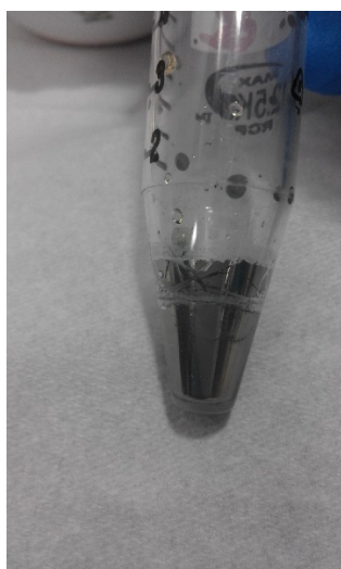
Figure S3: Reductive precipitation of palladium with ascorbic acid solution in water ( T = 25\text{ }^{\circ}\text{C} , 1\text{ mol L}^{-1} ascorbic acid).
