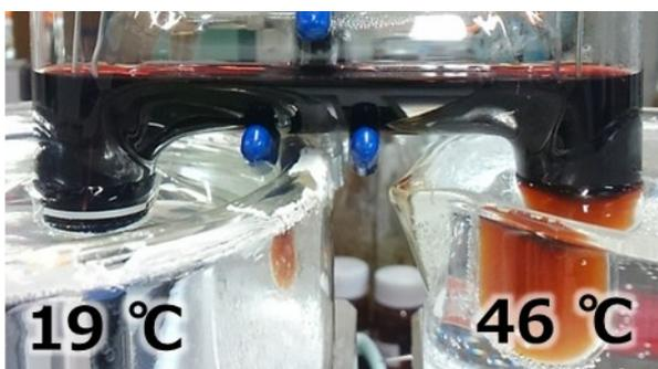
**Figure S2.** Photograph of thermocell.
