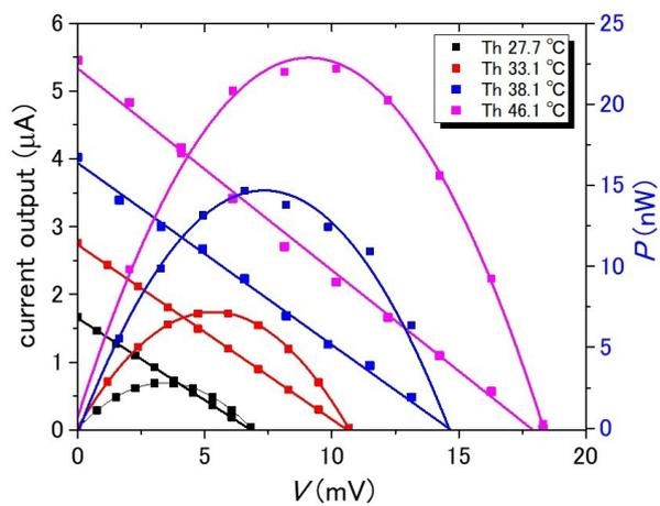
**Figure S9.** (a) I–V and P–V plots of a thermocell without a host at various temperatures at the hot electrode side. The temperature at the cold side was fixed at ca. 19.5 °C.
