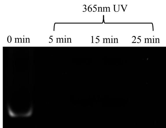
**Fig. S1** Study on cleavage performance of photocleavable linker (PC-linker) group by 18% PAGE
