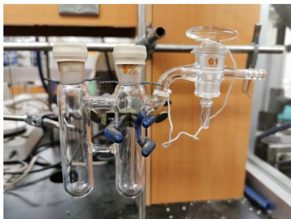
Two-chamber Schlenk tube (chamber I: left; chamber II: right)
