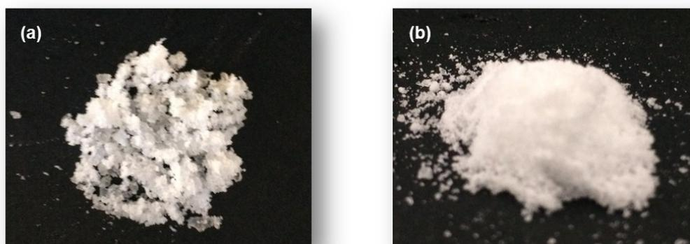
**Figure S3.** Appearance and rigidity of PEI snow with (a) 3.0 wt. %, (b) 6.0 wt. % of TTE. It was clear that higher levels of TTE could boost the powdery nature and increase the dryness of the PEI snow.
