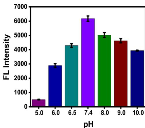
**Figure S5.** Effects of pH on the fluorescence of **4F-2CN-GSH** (100  $\mu\text{M}$ ) to GGT (300 U/L).  $\lambda_{\text{ex}} = 405$  nm.
