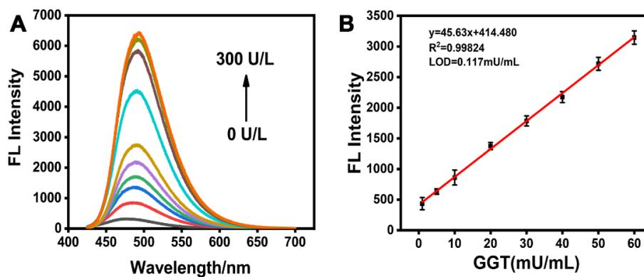
**Figure S6.** (A) Fluorescence spectral change of **4F-2CN-GSH** (100  $\mu\text{M}$ ) to GGT (0, 10, 20, 30, 40, 50, 100, 150, 250 and 300 U/L), and each spectrum was recorded after
