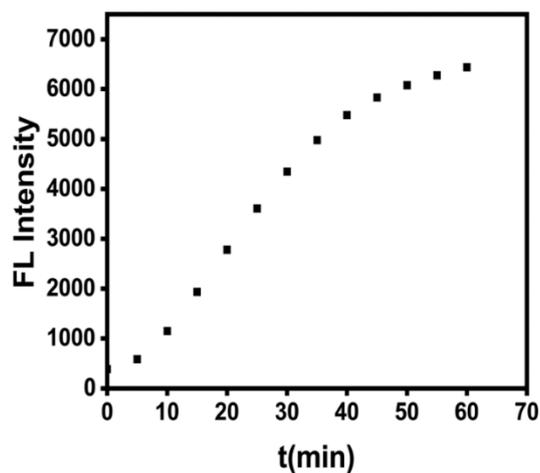
**Figure S4.** Time-dependent fluorescence intensity at 490 nm of **4F-2CN-GSH** (100  $\mu\text{M}$ ) to GGT (300 U/L).  $\lambda_{\text{ex}} = 405$  nm. Conditions: PBS (pH = 7.4, 10 mM) at 37  $^{\circ}\text{C}$ .
