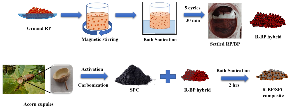
Scheme S1: Synthesis process of hybrid R-BP and hybrid R-BP/SPC composite
