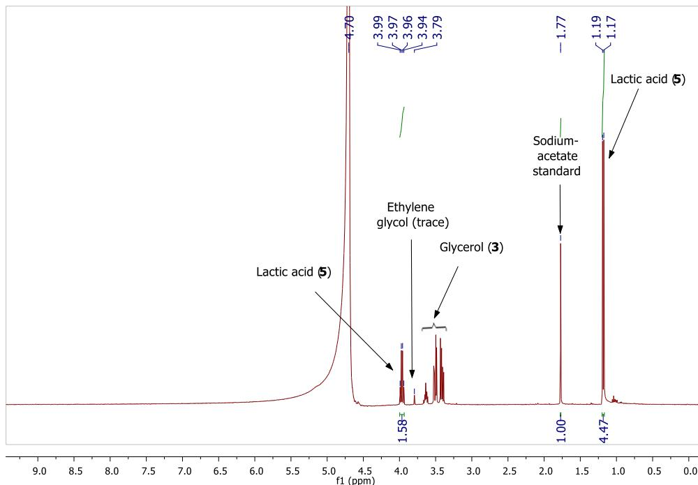
**Figure S19:**  $^1\text{H}$  NMR spectra of glycerol (**3**) dehydrogenation without solvent catalyzed by 0.03 mol% of **1c** (Table 2, entry 9).
