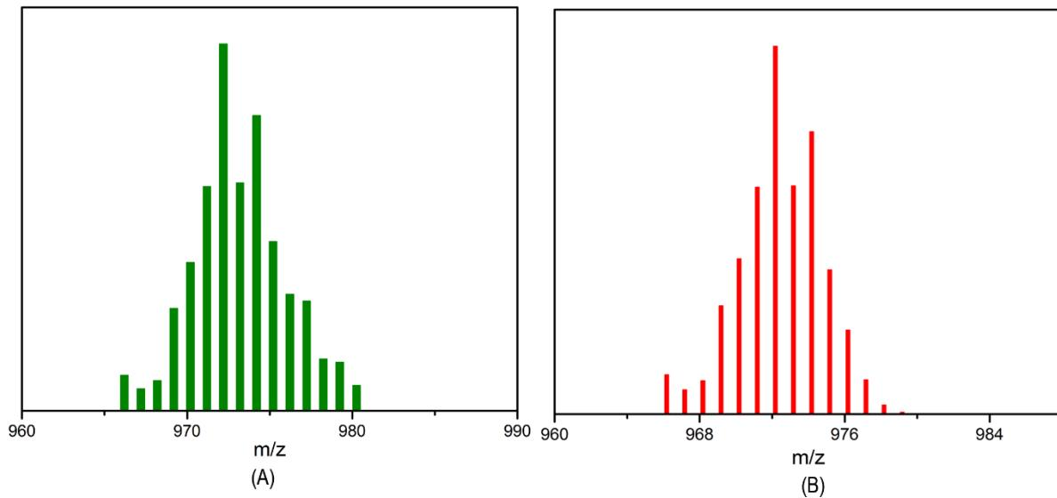
**Figure S4:** ESI-MS Expanded Spectra of Complex **1c** at  $m/z$  972.1952 (A) observed (B) Simulated
