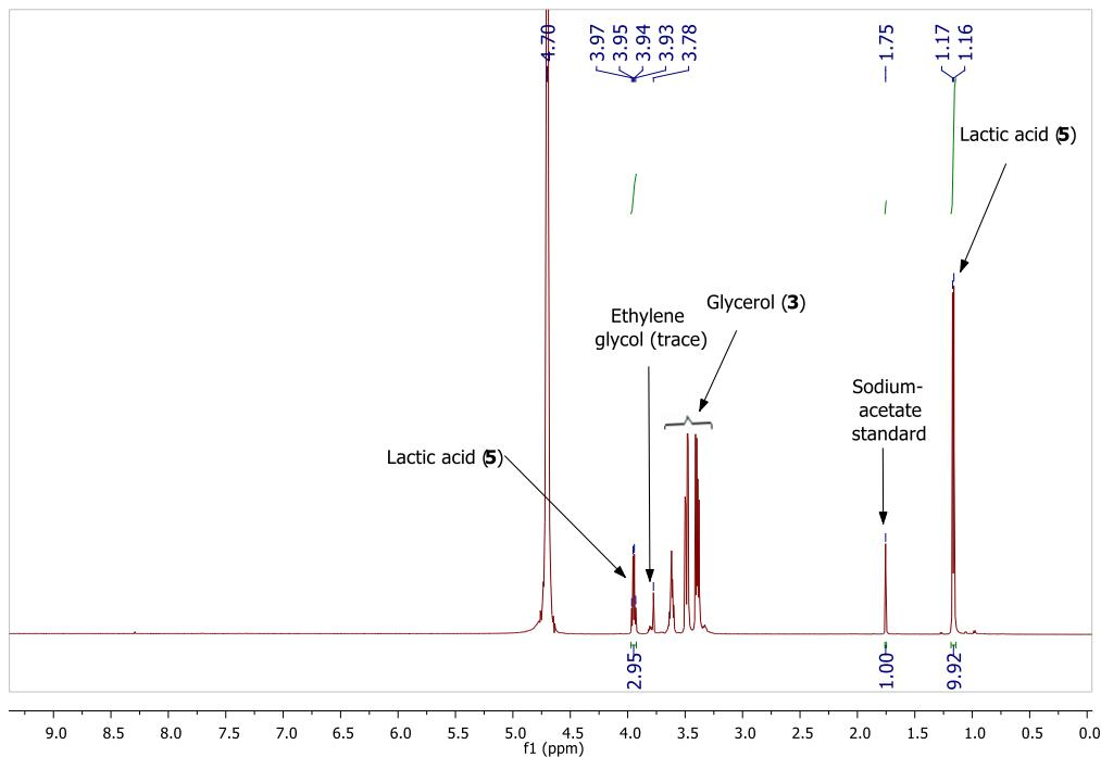
**Figure S15:**  $^1\text{H}$  NMR spectra of glycerol (**3**) dehydrogenation in water catalyzed by 0.03 mol% of **1c** (Table 2, entry 6).
