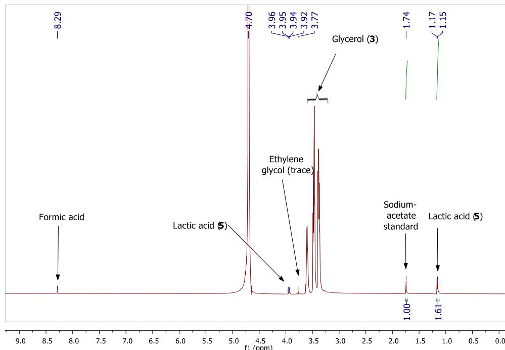
**Figure S22:** <sup>1</sup>H NMR spectra of glycerol (**3**) dehydrogenation in ethanol catalyzed by 0.003 mol% of **1c** (Table 2, entry 12).
