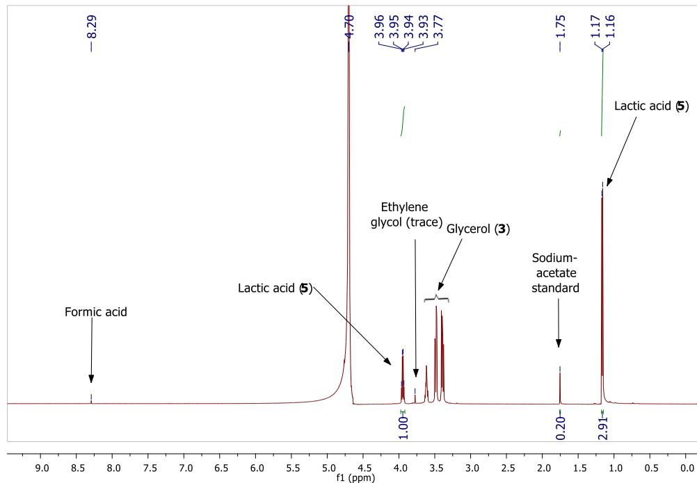
**Figure S24:**  $^1\text{H}$  NMR spectra of glycerol (**3**) dehydrogenation without solvent catalyzed by 0.003 mol% of **1c** (Table 2, entry 14).
