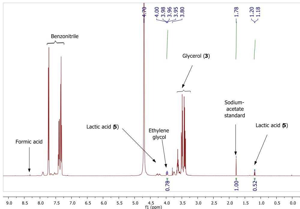
**Figure S14:**  $^1\text{H}$  NMR spectra of glycerol (**3**) dehydrogenation in benzonitrile catalyzed by 0.03 mol% of **1c** (Table 2, entry 5).
