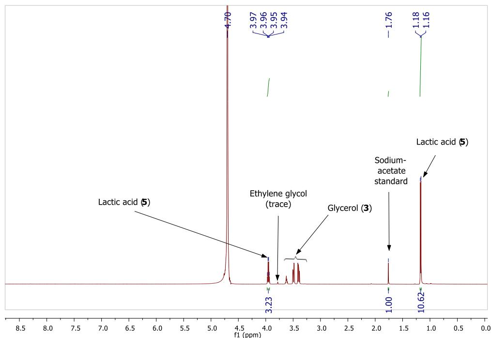
**Figure S10:** <sup>1</sup>H NMR spectra of glycerol (**3**) dehydrogenation catalyzed by 0.03 mol% [<sup>Bim2</sup>NNN]RuCl(PPh<sub>3</sub>)<sub>2</sub>]PF<sub>6</sub> (**1d**) (Table 1, entry 4).
