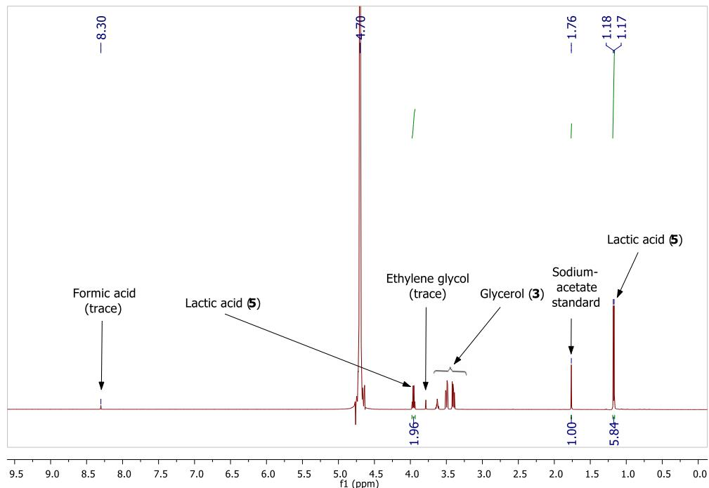
**Figure S7:** <sup>1</sup>H NMR spectra of glycerol (**3**) dehydrogenation catalyzed by 0.03 mol% (<sup>t</sup>Bu<sub>2</sub>NNN)RuCl<sub>2</sub>(PPh<sub>3</sub>) (**1a**) (Table 1, entry 1).
