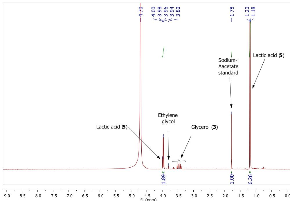
**Figure S18:** <sup>1</sup>H NMR spectra of glycerol (3) dehydrogenation in ethanol catalyzed by 0.03 mol% of **1c** (repeat reaction, Table 2, entry 8).
