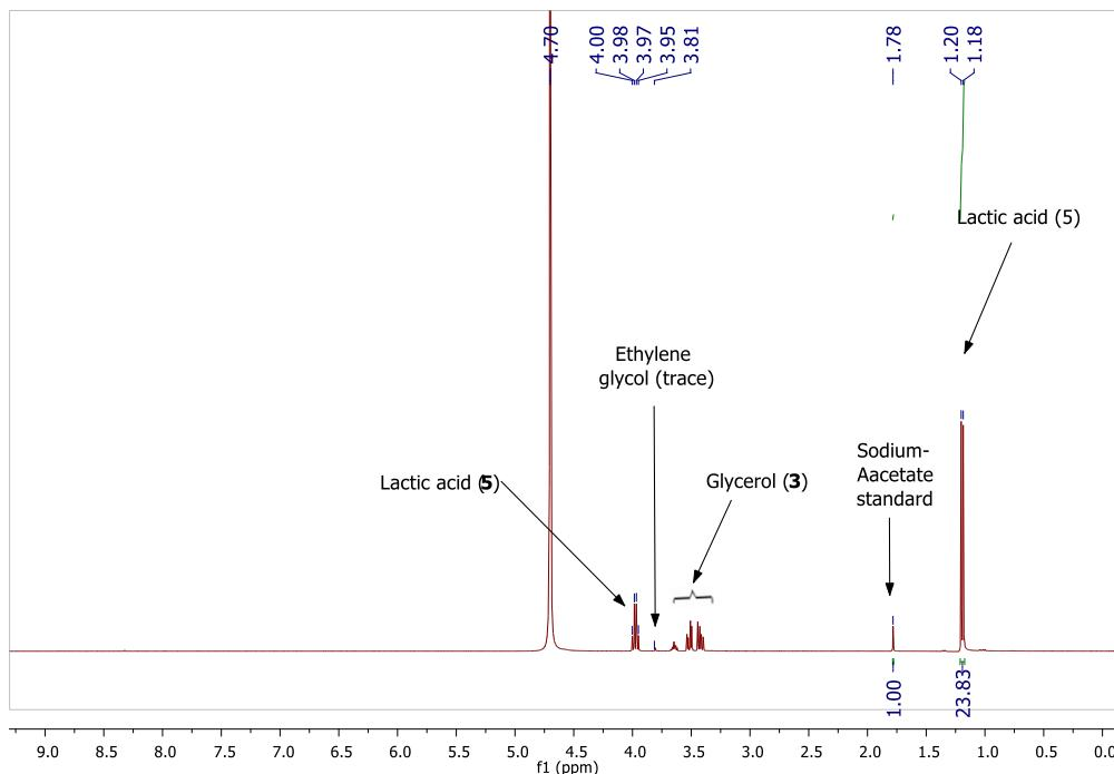
**Figure S20:**  $^1\text{H}$  NMR spectra of glycerol (**3**) dehydrogenation in dioxane catalyzed by 0.03 mol% of **1c** (Table 2, entry 10).
