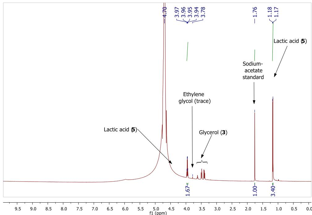
**Figure S13:**  $^1\text{H}$  NMR spectra of glycerol (**3**) dehydrogenation in *p*-xylene catalyzed by 0.03 mol% of **1c** (Table 2, entry 4).
