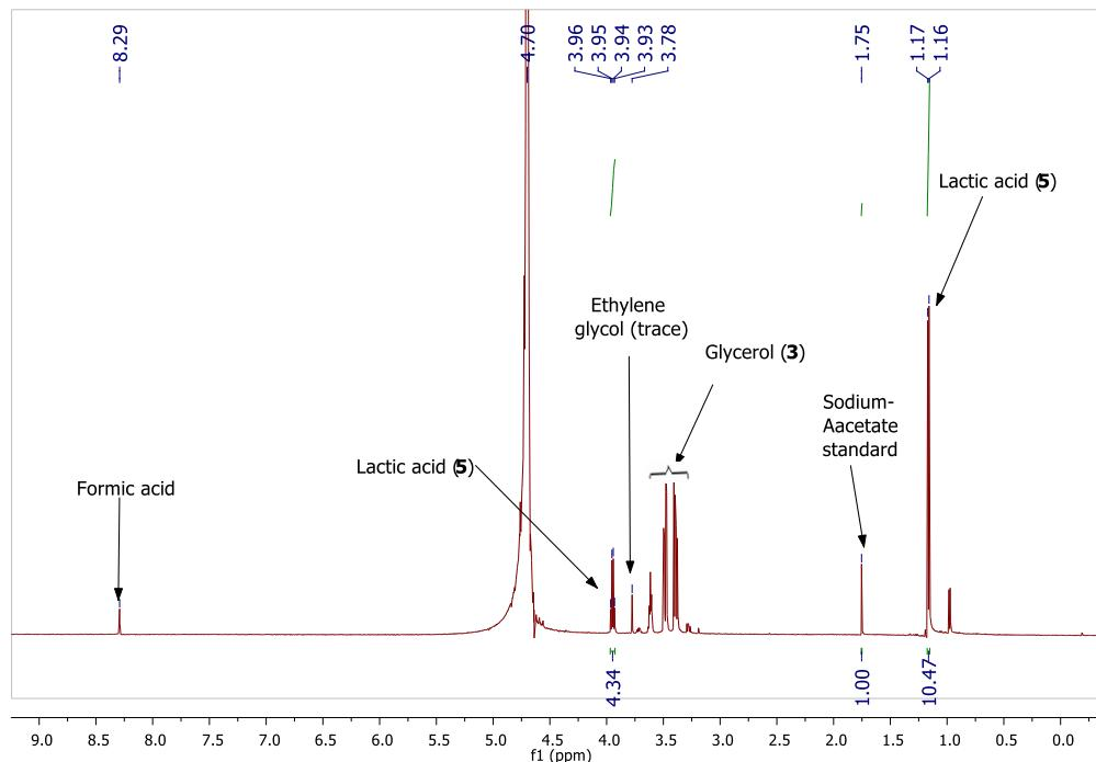
**Figure S21:** <sup>1</sup>H NMR spectra of glycerol (**3**) dehydrogenation in ethanol catalyzed by 0.03 mol% of **1c** (Table 2, entry 11).
