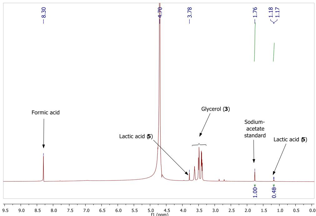
**Figure S12:**  $^1\text{H}$  NMR spectra of glycerol (**3**) dehydrogenation in DMF catalyzed by 0.03 mol% of **1c** (Table 2, entry 3).
