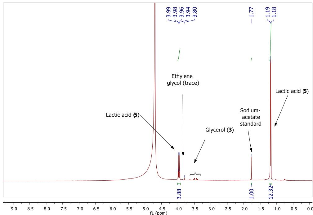
**Figure S17:** <sup>1</sup>H NMR spectra of glycerol (3) dehydrogenation in ethanol catalyzed by 0.03 mol% of **1c** (Table 2, entry 8).
