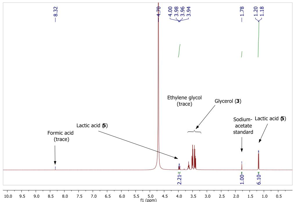
**Figure S8:** <sup>1</sup>H NMR spectra of glycerol (**3**) dehydrogenation catalyzed by 0.03 mol% (Ph<sub>2</sub>NNN)RuCl<sub>2</sub>(PPh<sub>3</sub>) (**1b**) (Table 1, entry 2).
