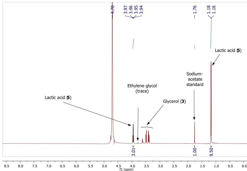
**Figure S9:** <sup>1</sup>H NMR spectra of glycerol (**3**) dehydrogenation catalyzed by 0.03 mol% [<sup>Bim2</sup>NNN]RuCl(PPh<sub>3</sub>)<sub>2</sub>]Cl (**1c**) (Table 1, entry 3).
