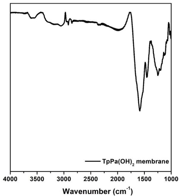
**Fig. S1** FT-IR spectrum of the TpPa(OH)<sub>2</sub> membrane.
