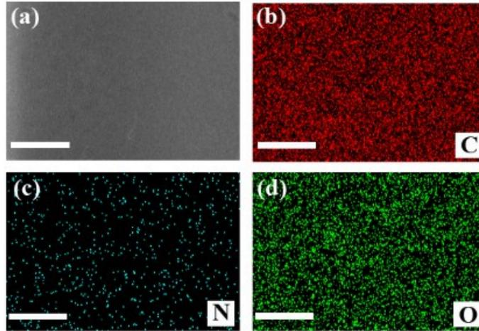
**Fig. S3** (a) SEM image and (b-d) element mappings of the  $\text{TpPa}(\text{OH})_2$  membrane (scale bar:  $10\ \mu\text{m}$ ).
