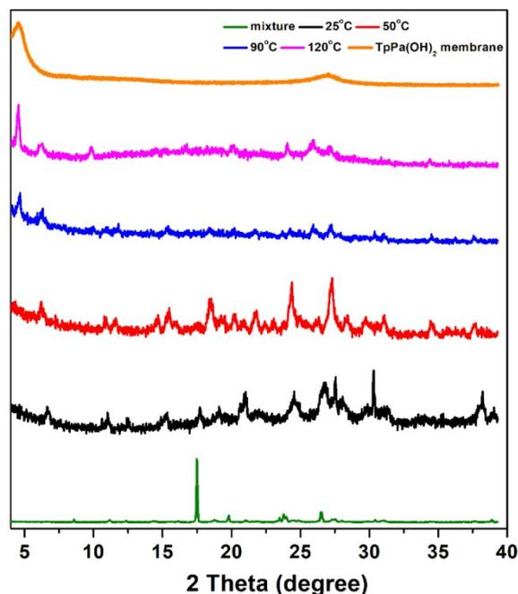
**Fig. S10** PXR D patterns of the TpPa(OH)<sub>2</sub> membrane during the growth process (green: mixture of Tp, Pa(OH)<sub>2</sub> and PTSA, black: precursor (the above mixture after homogenisation with water), red: precursor after heating for 6 h at 50 °C, blue: precursor after another heating for 6 h at 90 °C, purple: precursor after additional heating for 6 h at 120 °C, orange: membrane after washing with water, THF, acetone).
