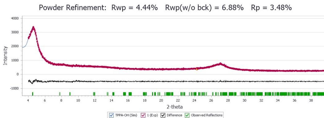
**Fig. S2** Pawley refinement of XRD for the TpPa(OH)<sub>2</sub> membrane. Pawley refinement indicates the agreement between simulated and experimental PXRD patterns.
