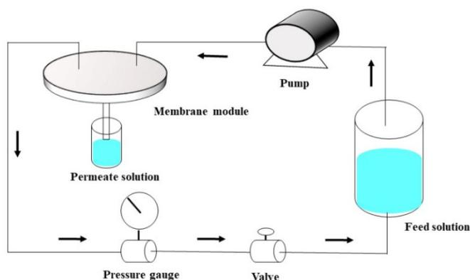
**Fig. S11** A scheme for the setup of RO separation for water desalination.
