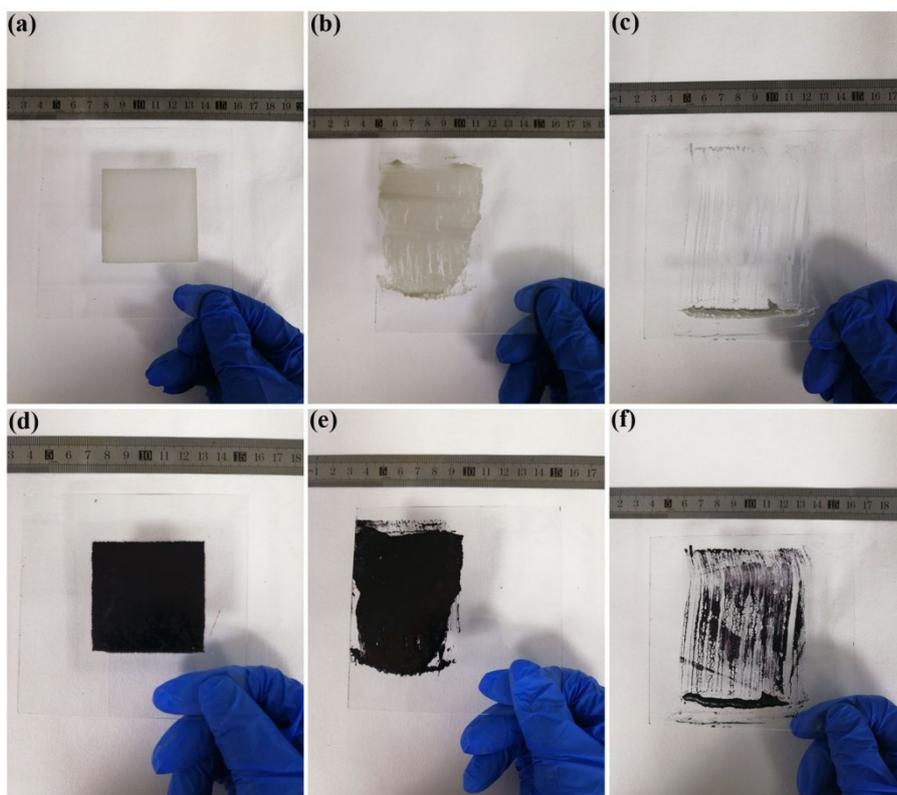
**Fig. S6** (a-c) Optical photos of the TpPa(OH)<sub>2</sub> precursors prepared by different methods (a: screen printing, b: glass casting, c: knife casting), and (d-f) optical photos of correspondingly obtained membranes after heating (50 °C-90 °C-120 °C).
