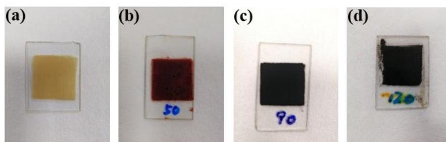
**Fig. S9** (a-d) Optical photos of the TpPa(OH)<sub>2</sub> membrane at each temperature during the growth process.
