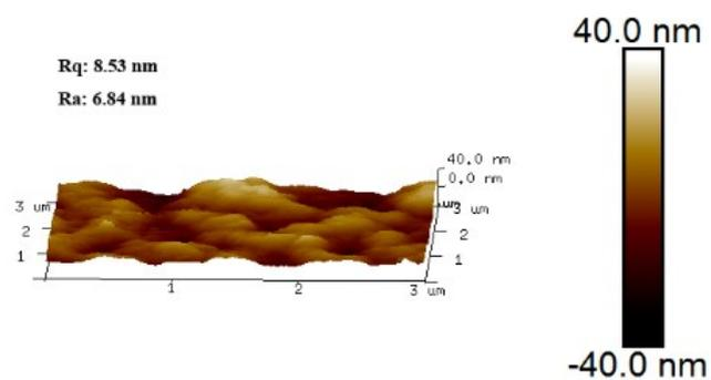
**Fig. S5** AFM image of the TpPa(OH)<sub>2</sub> membrane.
