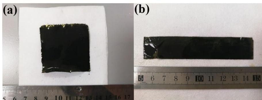
**Fig. S8** (a, b) Optical photos of the synthesised TpPa(OH)<sub>2</sub> membranes with two different sizes.
