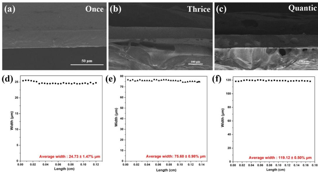
**Fig. S4** (a, b, c) Cross-section SEM images of  $\text{TpPa}(\text{OH})_2$  membranes with  $25\ \mu\text{m}$  (once),  $76\ \mu\text{m}$  (thrice) and  $119\ \mu\text{m}$  (quantic) in thickness, respectively; (d, e, f) the corresponding thicknesses at different positions along the length of the  $\text{TpPa}(\text{OH})_2$  membrane (the thickness is reported in average width with relative standard deviation).
