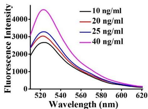
**Fig. S6.** Fluorescence emission spectra in response to the same amounts of total nuclear extract (0.25mg/ml) treated by different concentrations of TNF- $\alpha$ . The concentration of TF-binding probe is 500 nM.
