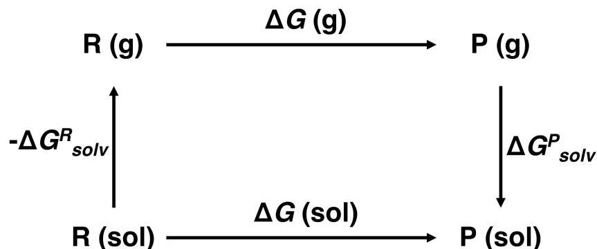
Scheme S2. Thermodynamic cycle utilized for calculation of reduction potentials.
