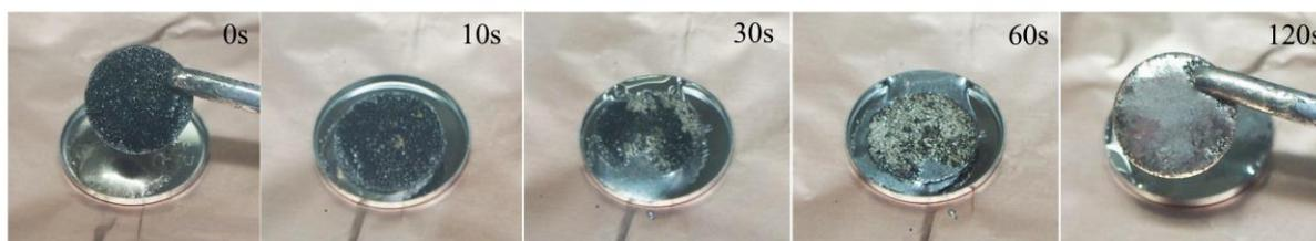
**Figure S2** Time-lapse images of Li melt-infusion process into GO-Ni composite (conducted at a heating platform, 300 °C).
