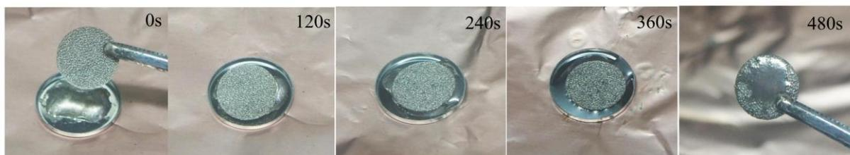
**Figure S1** Time-lapse images of Li melt-infusion process into Ni foam (conducted at a heating platform, 300 °C).
