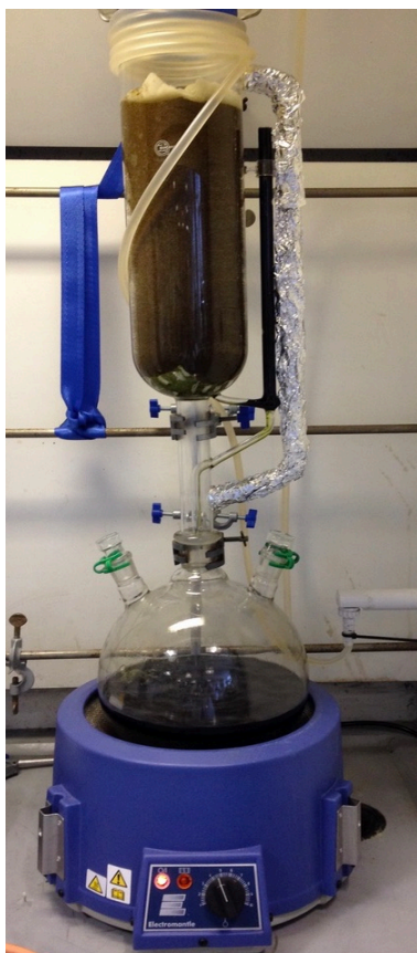
Figure S1: Equipment used in large-scale Soxhlet extraction. A) Large-scale Soxhlet extraction of bay leaves into a 5L round-bottomed flask. B) Partial purification of undecaprenol by flash column-chromatography. Column diameter is 10 cm and height is 45 cm.
