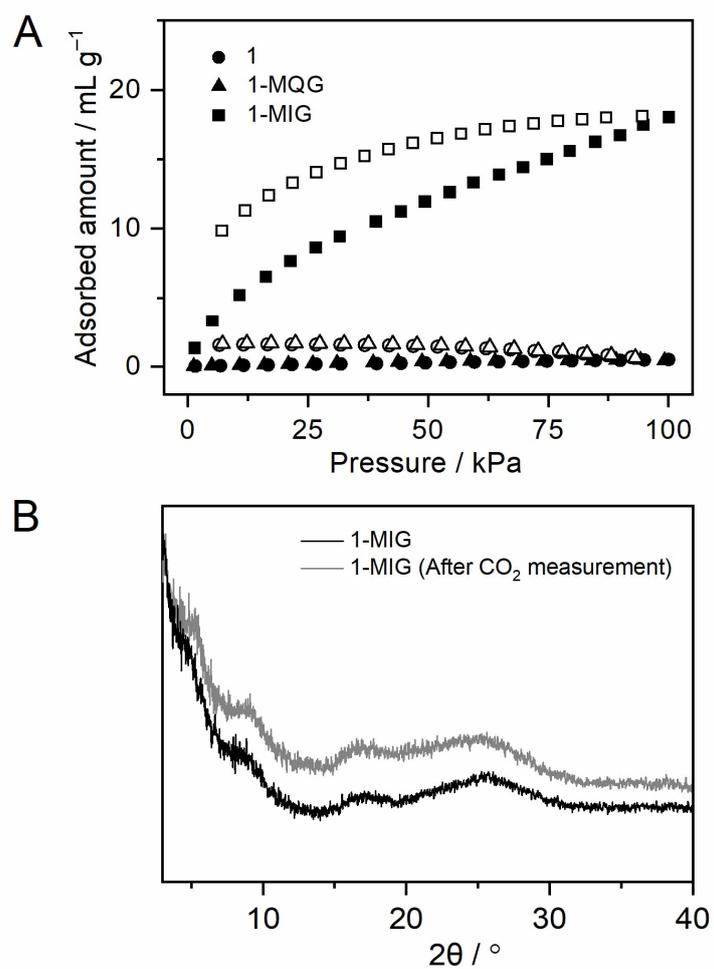
**Fig. S10.** (A) CO<sub>2</sub> adsorption and desorption isotherms of **1**, **1-MQG** and **1-MIG** at  $-78.15$  °C. (B) PXRD patterns of **1-MIG** before and after CO<sub>2</sub> adsorption and desorption isotherm measurements.
