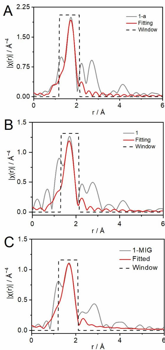
**Fig. S3.** Radial distribution functions of **1-a**, **1** and **1-MIG** (gray) and fitting curve (red) at room temperature.
