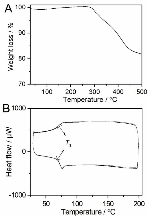
**Fig. S5.** (A) TGA profile of **1-MQG** under  $\text{N}_2$ . (B) DSC profiles (6 cycles) of **1-MQG**. Scan rates were  $10\text{ }^\circ\text{C min}^{-1}$ .
