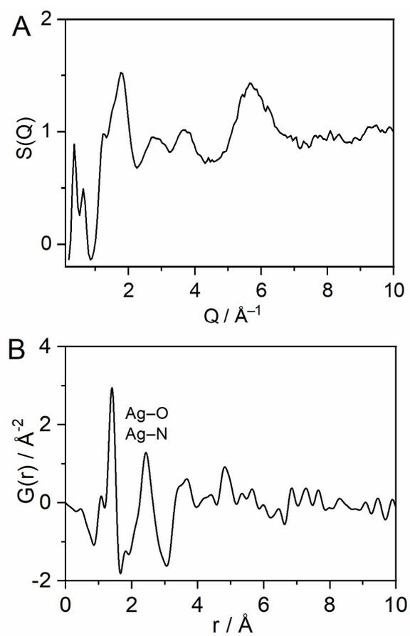
**Fig. S9.** (A) X-ray total structure factor  $S(Q)$  (B) Reduced pair distribution function (PDF) profiles of 1-MIG.
