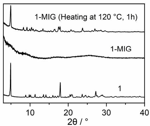
**Fig. S8.** PXRD patterns of 1, 1-MIG, 1-MIG after heating at 120 °C for 1 h.
