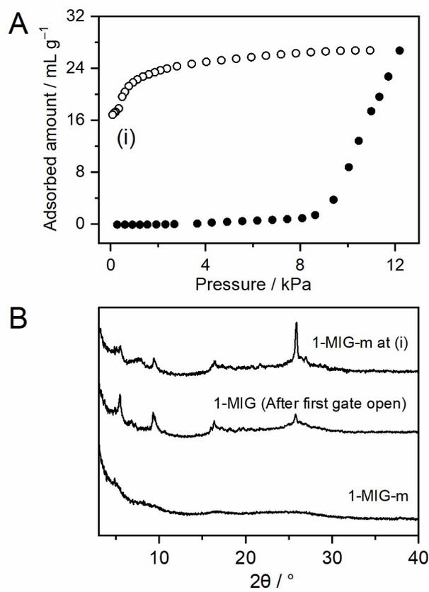
**Fig. S12.** (A) Benzene vapour sorption study of **1-MIG-m** at 25 °C. (B) PXRD patterns of **1-MIG-m** after benzene sorption measurement (top) and **1-MIG** after first gate open (second from top).
