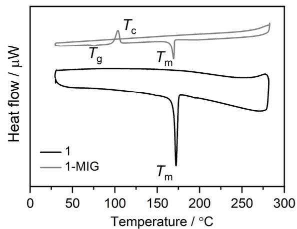
**Fig. S6.** DSC profiles of **1** and **1-MIG** up to 280  $^{\circ}\text{C}$  under  $\text{N}_2$ . Scan rate were 10  $^{\circ}\text{C min}^{-1}$ .
