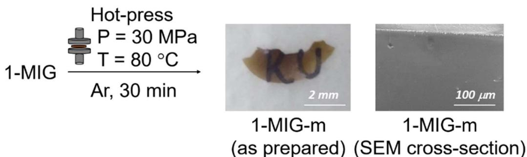
**1.5. Preparation of crystal-glass hierarchical structure:** The crystal-glass hierarchical structure was prepared after soaking of **1-MIG-m** (2 mm diameter and 0.3 mm of thick) at 25 °C in anhydrous benzene for 24 h and dried under Ar for 12 h. Surface morphology of **1-MIG-m** before (left) and after (right) benzene soaking in Ar atmosphere characterized by SEM.
