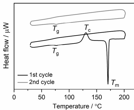
**Fig. S7.** DSC profiles of the hand-grinded **1-MQG** under  $\text{N}_2$ . Scan rates were 10  $^{\circ}\text{C min}^{-1}$ .
