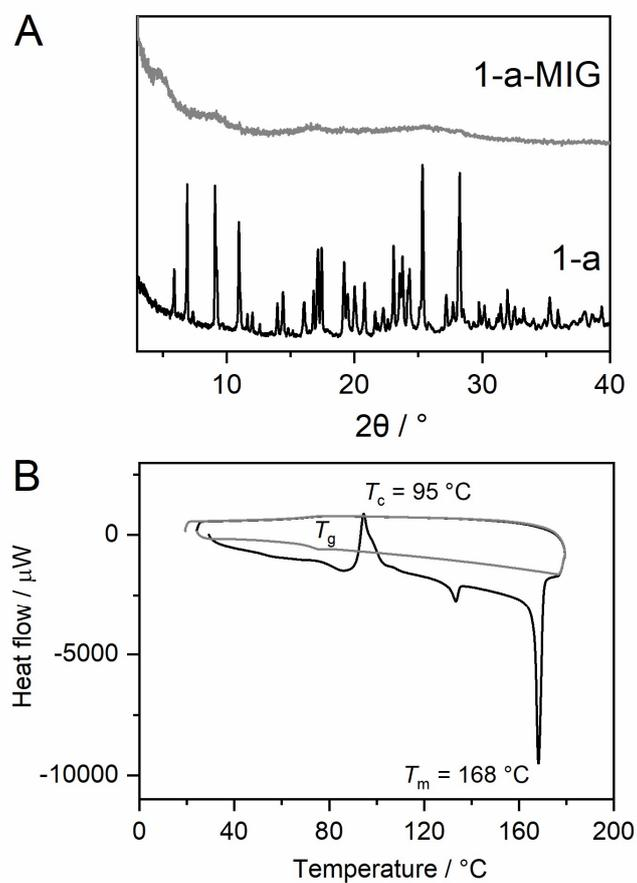
**Fig. S13.** (A) PXR D patterns of **1-a** and **1-a-MIG**. (B) DSC profile of **1-a-MIG** up to 280 °C under N<sub>2</sub>. Scan rates were 10 °C min<sup>-1</sup>.
