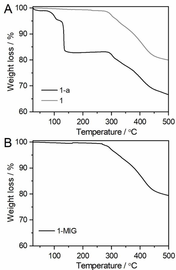
**Fig. S1.** (A) TGA profiles of **1-a** and **1**. (B) TGA profile of **1-MIG**. Measurements were carried out under N<sub>2</sub> atmosphere. Scan rates were 10 °C min<sup>-1</sup>.
