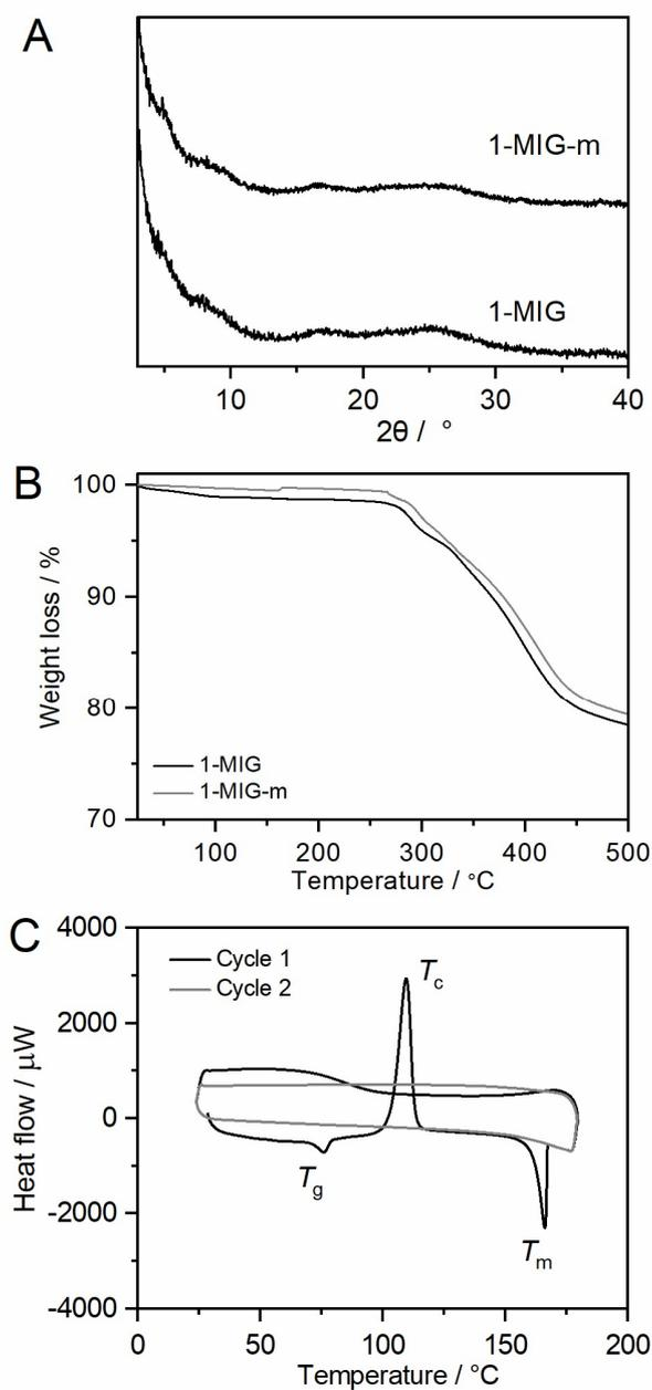
**Fig. S11.** (A) PXR D patterns of **1-MIG** and **1-MIG-m**. (B) TGA profiles of **1-MIG** and **1-MIG-m**. Scan rates were  $10\text{ }^\circ\text{C min}^{-1}$ . (C) DSC profiles for **1-MIG-m** (2 cycles).  $T_g$ ,  $T_m$  and  $T_c$  represent the glass transition, crystallization and melting temperatures. Scan rates were  $10\text{ }^\circ\text{C min}^{-1}$ .
