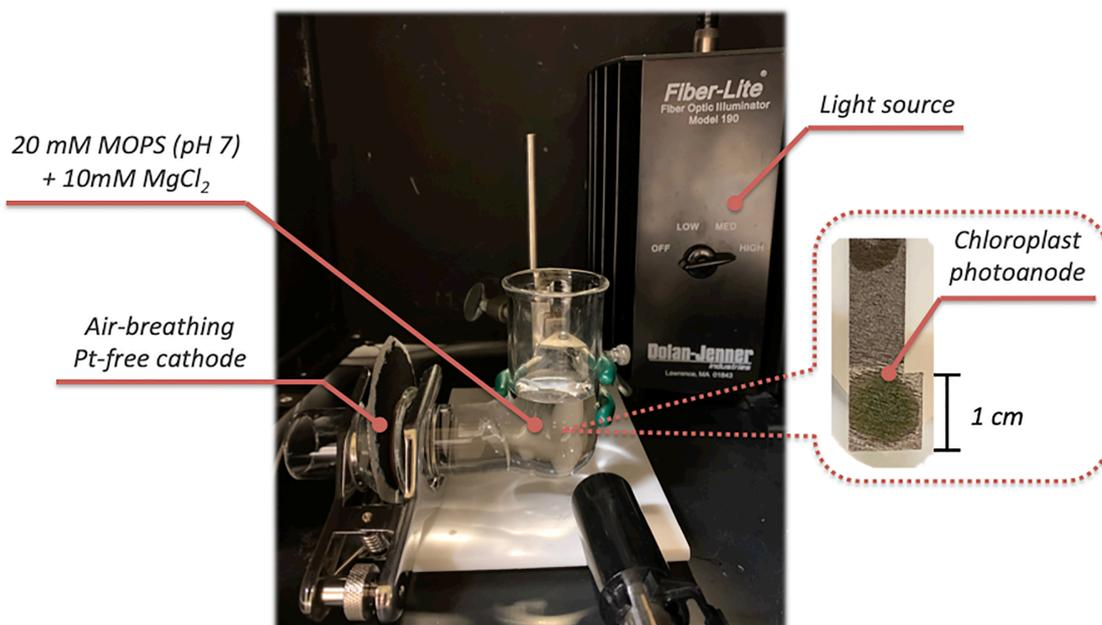
Fig. S1 Components of the chloroplast biosolar cell. The callout shows the chloroplast photoanode with immobilized chloroplasts (green area).
