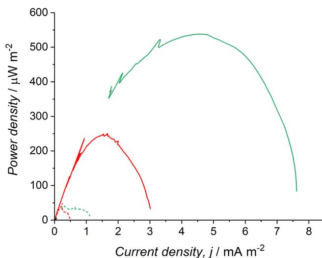
**Fig. S4** Power density under illumination (continuous lines) and dark (dashed lines) for EGDGE-modified (green) and regular (red) chloroplast biosolar cells. Control cells with abiotic photoanodes (black).
