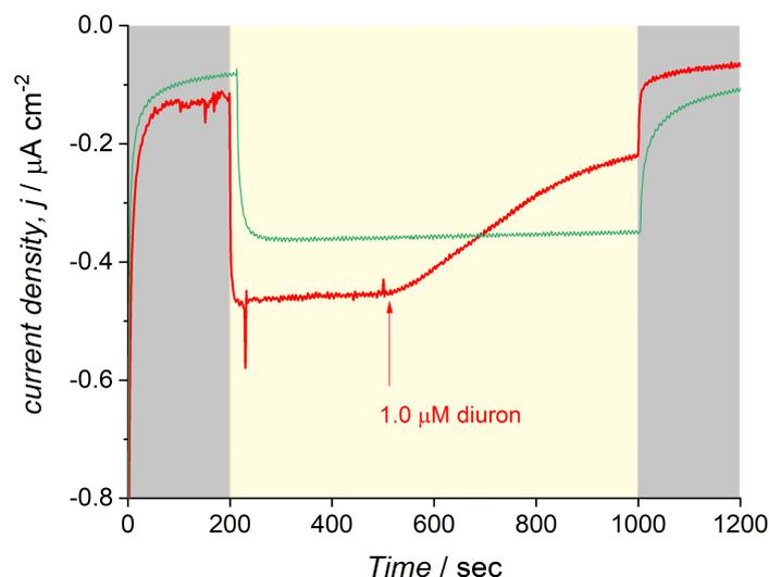
**Fig. S3** Representative amperometric *i-t* curves for a EGDGE-modified chloroplast photoanode with 1.0  $\mu\text{M}$  diuron addition at 500 sec (red line) and for the same photoanode after being in a diuron-free solution for 1 hour (green line). Yellow background indicates light conditions.
