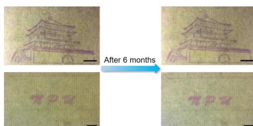
Figure S20. Photographs of the inkjet-printed fluorescent pattern on day 1 and after 6 months. The printed pattern derived from G1/TCNB features enough stability, as evidenced by unchanging of the emission color under the ambient conditions for at least 6 months.
