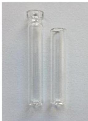
**Figure S2.** Left: uncrimped vial; right: vial after removal of the headspace section.
