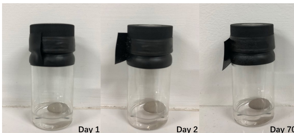
Fig. S4 Chemical stability of the ETFA electrolyte with Li metal tested through immersing Li metal in the electrolyte for days.
