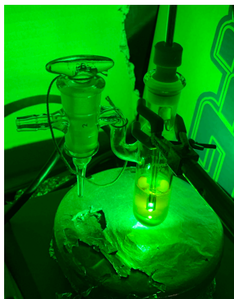
Figure S3. Experiment set-up image of photo-driven the dyad ( C1 ) catalyzed the reaction using halogen lamp ( \lambda_{\geq 520\text{ nm}} ) or LED ( \lambda_{\text{max}}=521\text{ nm} ).
